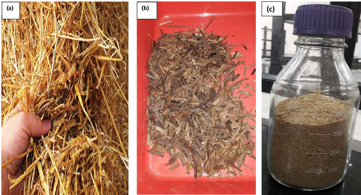
Figure 3.1. (a) Rice straw obtained from a local farm (b) Dried rice straw in Hot air oven (c) Grinded Rice Straw stored in a Duran bottle
