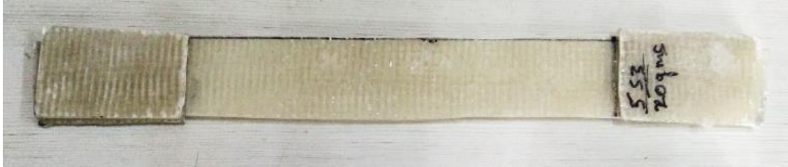
Figure 4.2 A tensile testing specimen of glass epoxy composite laminate (GFRP) as per ASTM D3039
