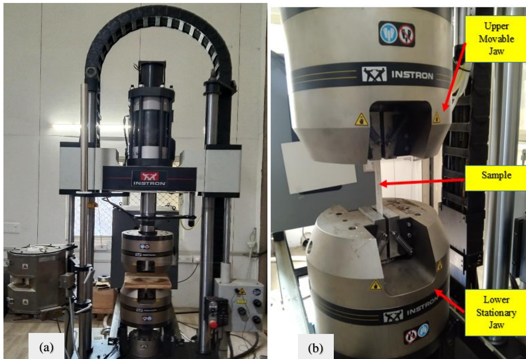
Figure 3.5 Test Setup (a) Dynamic UTM (b) Specimen mounted in Dynamic UTM for fatigue test (Courtesy: IIT, Mandi)
