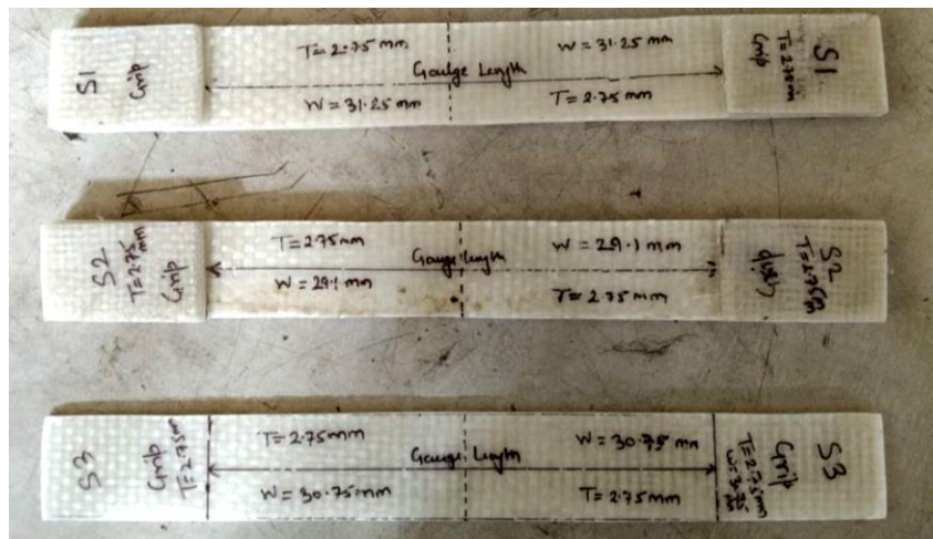
Figure 4.7 GFRP Specimen for fatigue testing under tension-tension loading with 2 Hz frequency
