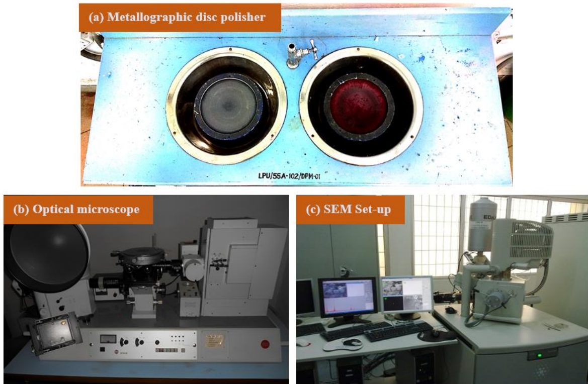
Figure 4.9: Set Up for Metallurgical and Microscopic Studies: (a) Metallographic disc polisher (Courtesy: Lovely Professional University, Punjab); (b) Optical microscope and (c) SEM Set-up (Courtesy: IIT, Roorkee)
