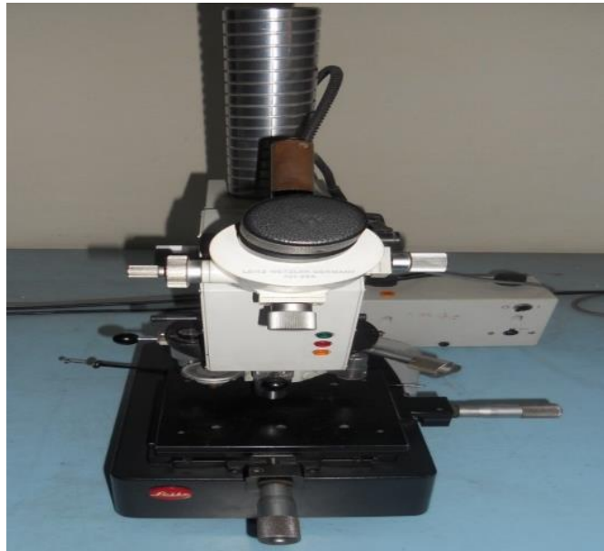
Figure 4.10: Vickers Microhardness Test Set-Up for Hardness Test (Courtesy: IIT, Roorkee)
