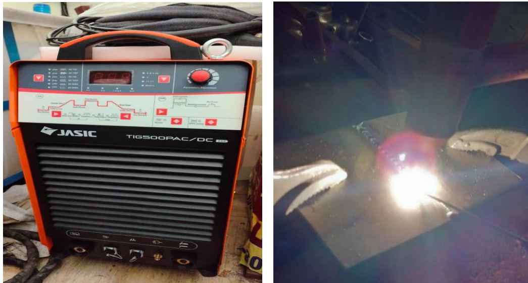
Figure 4.4: Welding Machine Set-up and Welding Process
