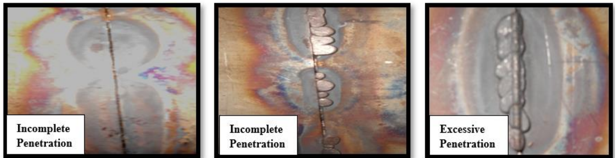
Figure 4.5: Improper Weld Bead Profiles of Pilot Weld Samples
