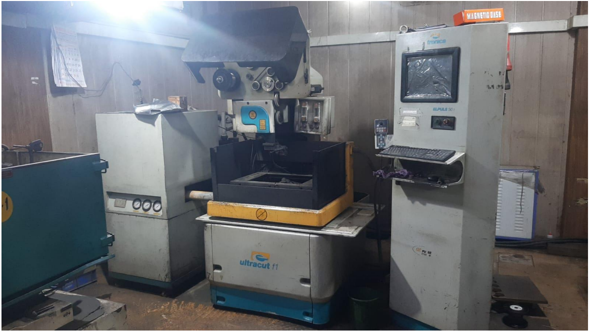
Figure 4.7: Wire Cut Electron Discharge Machining Set-Up
