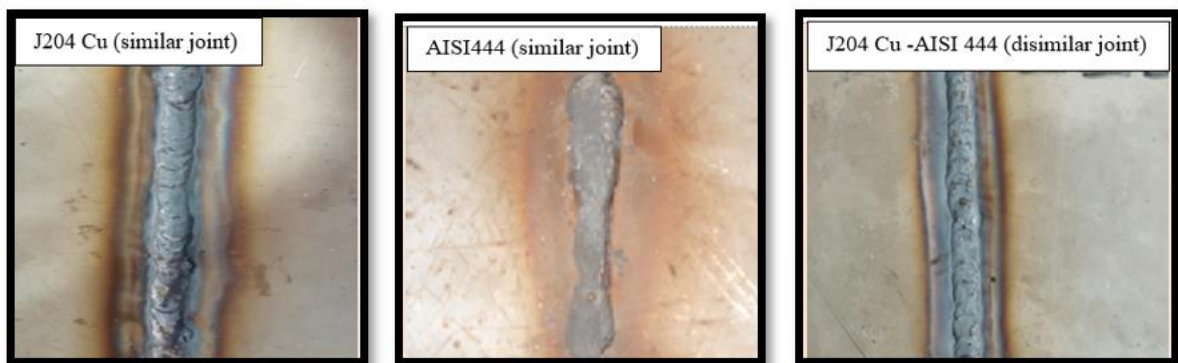
Figure 4.6: Final Weld Joints
