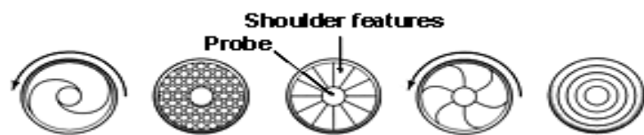
Figure 2.4: Pictorial view of Friction Stir Welded tools Shoulder profile.
