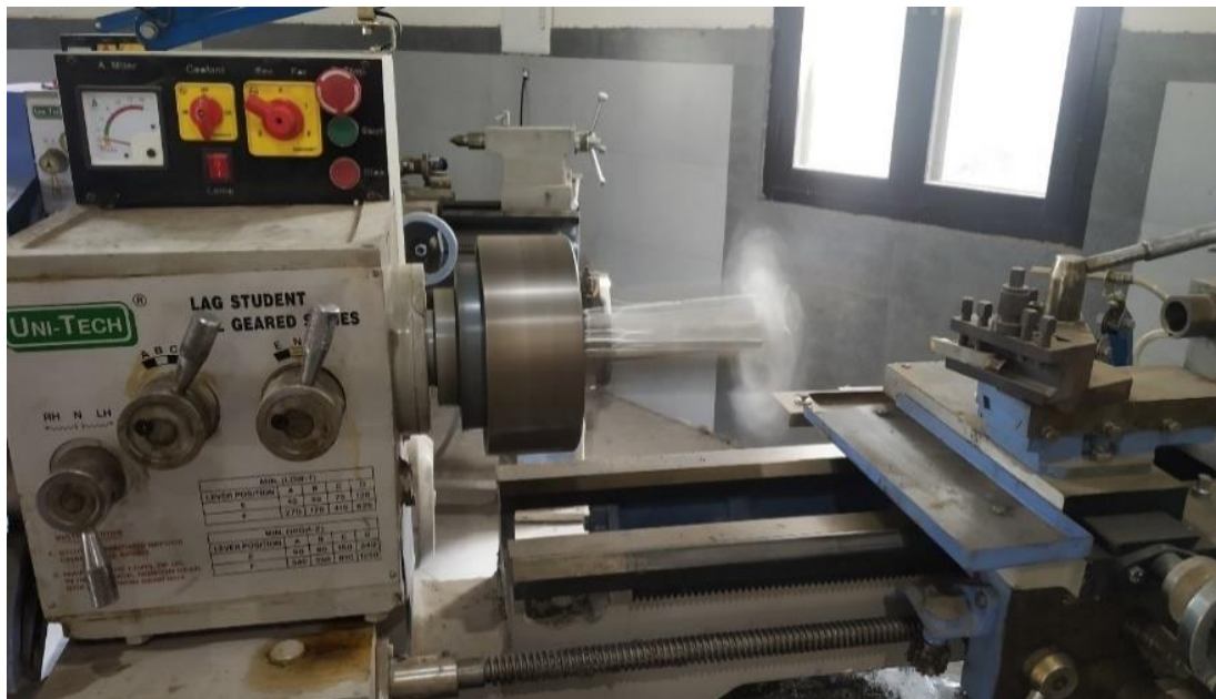
Fig. 3.2 Mixing of powder (90wt% HA and 10wt% \text{ZrO}_2 ) on lathe machine.
