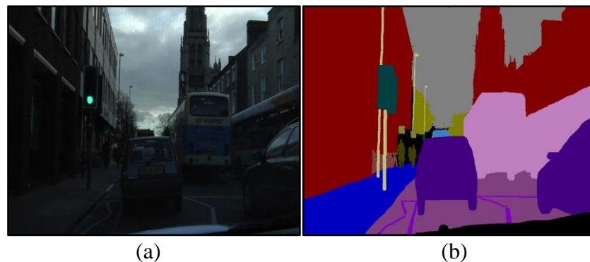
Figure 3.12 (a) A sample of a frame taken from the CamVid dataset, (b) An example of a frame labeled on a pixel-by-pixel basis from the CamVid dataset.
