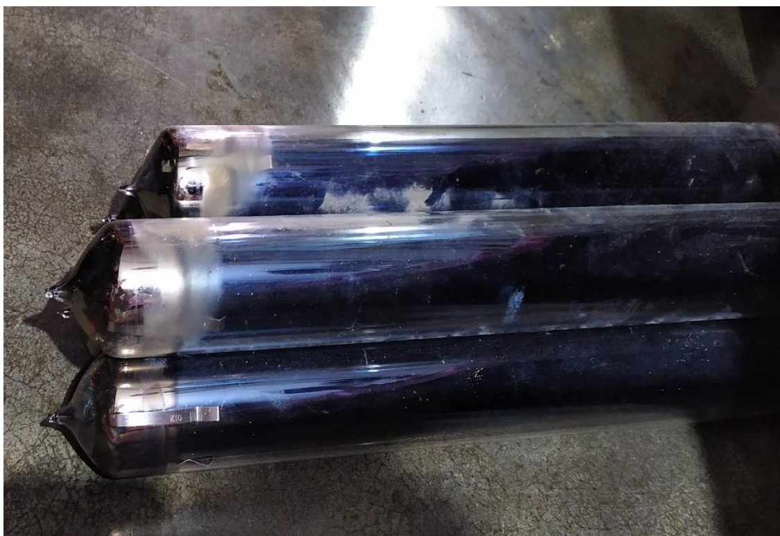
Figure 3.8 b. Photographic view of Evacuated Tube
