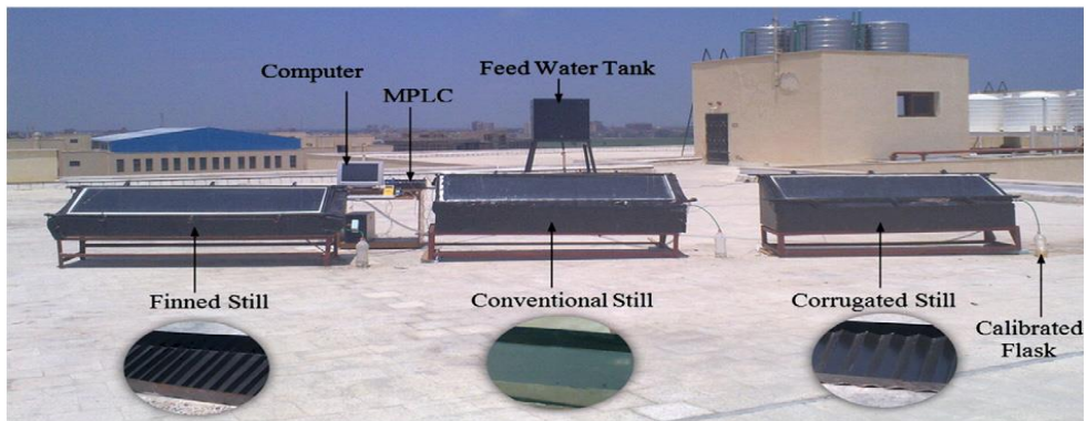
Figure 2.11. Schematic view of absorbing materials in the solar still. [40]
