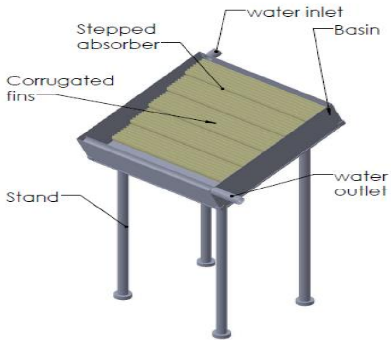
Figure 3.3. Schematic diagram of experimental setup without evacuated tube
