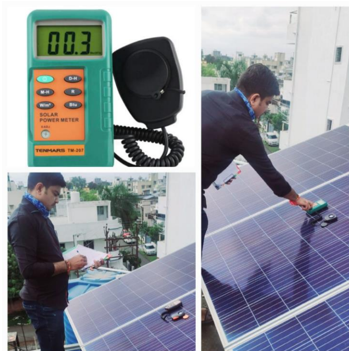
Fig. 4.9: Measurement of irradiance using solar meter
