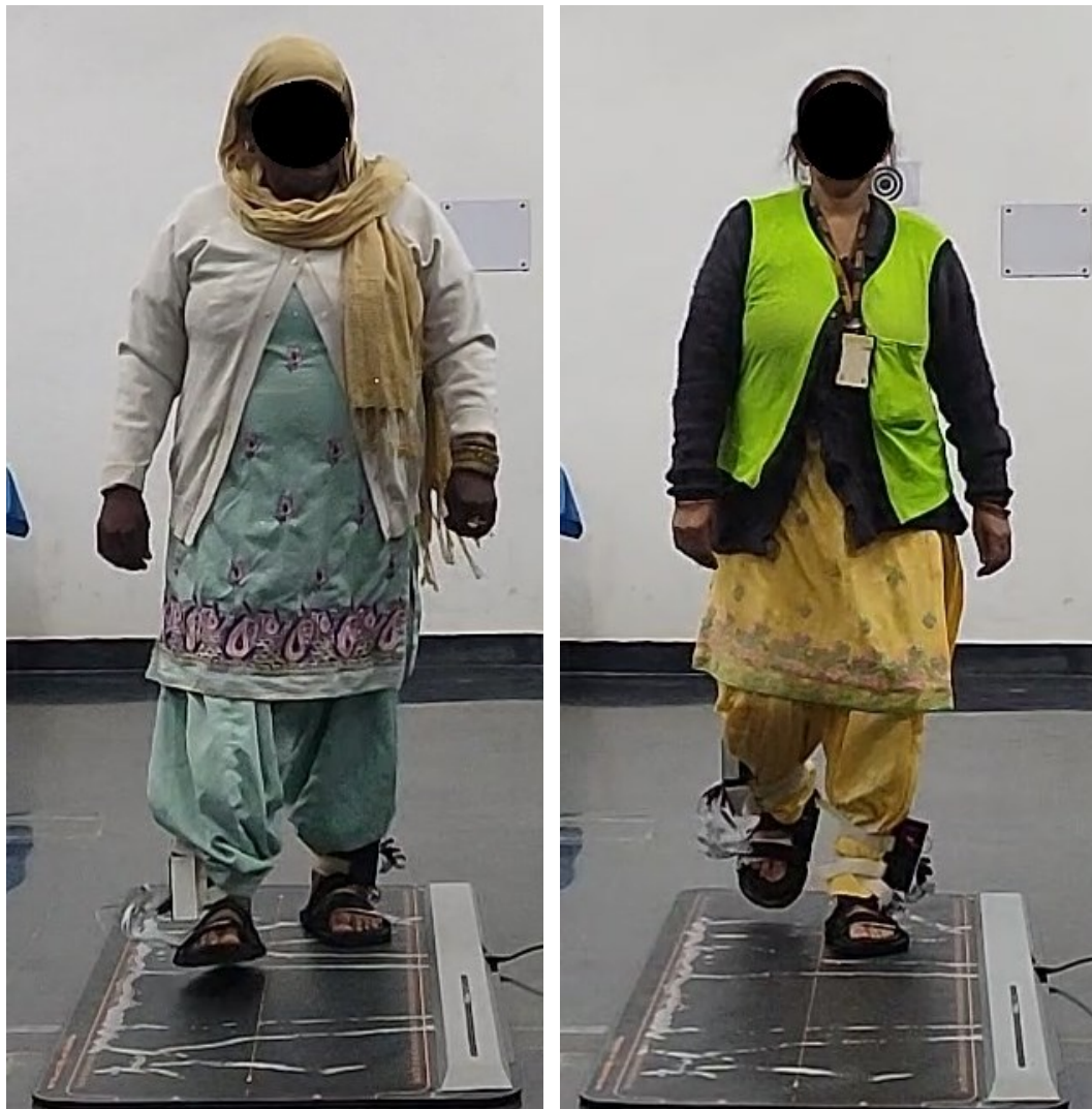
Figure 3. 14 Application of DT-walk device on patient's leg while standing on WinTrack platform for validity and reliability testing of DT-walk while walking.
