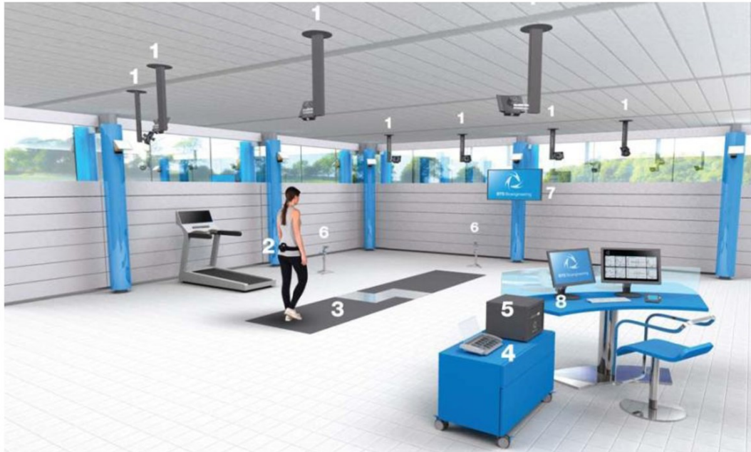
Figure 2. 3 BTS Gait Lab configuration. (1) infrared video cameras; (2) inertial sensor; (3) GRF measurement walkway; (4) wireless EMG; (5) workstation; (6) video recording system; (7) TV screen; (8) control station.
