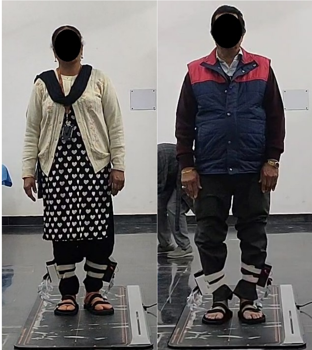
Figure 3. 13 Application of DT-walk device on patient's leg while standing on WinTrack platform for validity and reliability testing of DT-walk in standing position.
