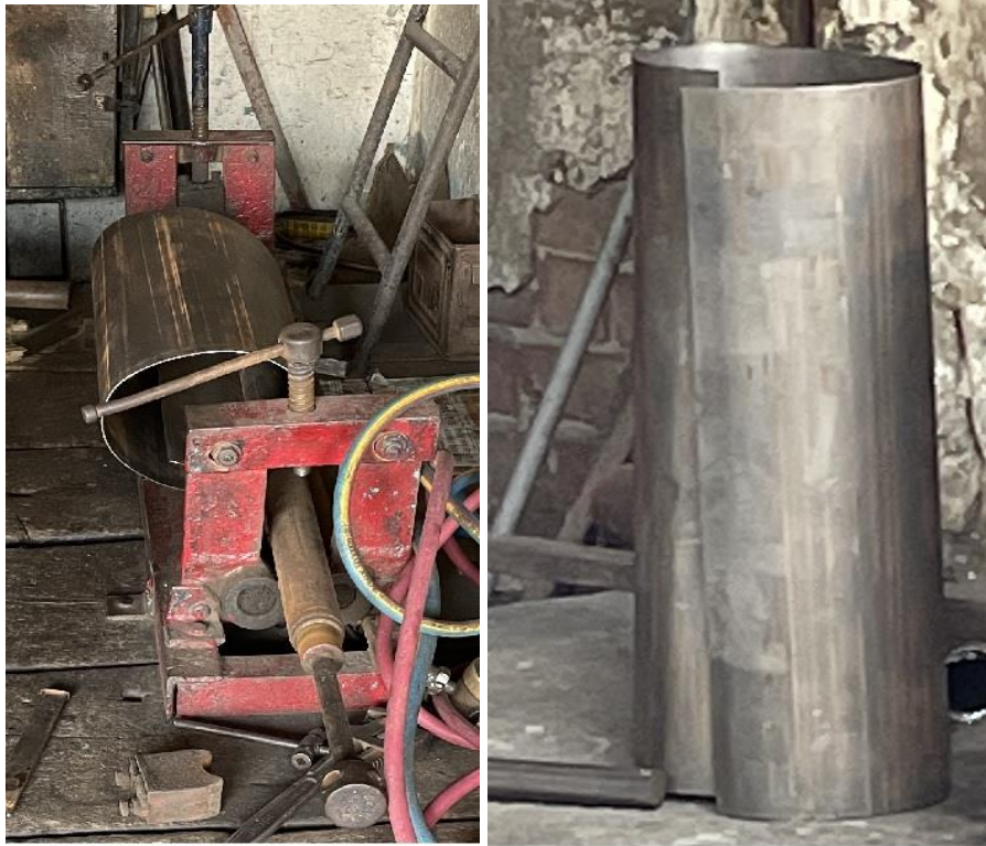
Figure 6.11. (a) Sheet in rolling machine, (b) rectangular sheet after rolling
