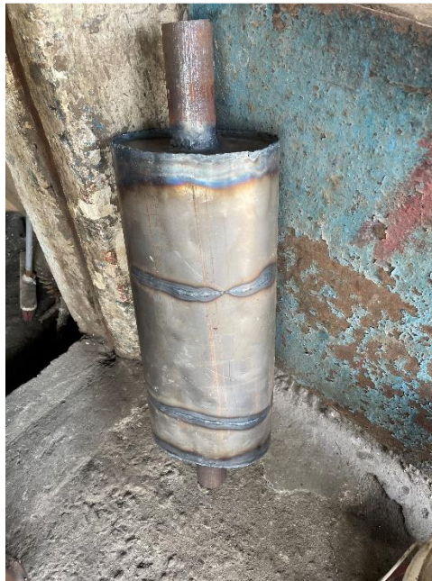
Figure 8.14 Hybrid muffler after welding all components
