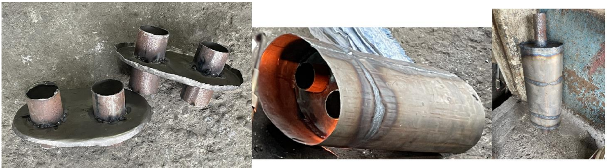
Figure 6.12. Fabrication process of existing muffler with the baffles and tubes placed inside muffler
