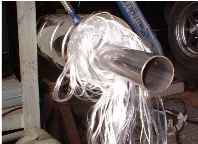
Figure 1.7. Dissipative muffler (Source: Silex Exhaust Silencers, Inc.)
