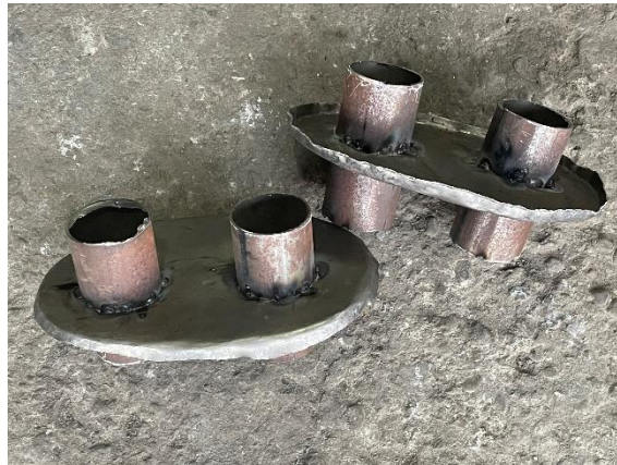
Figure 6.9. Baffle plates with tubes
