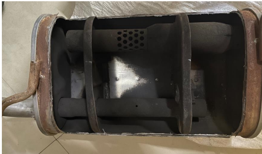
Figure 1.6. Reactive muffler of WagonR [41]
