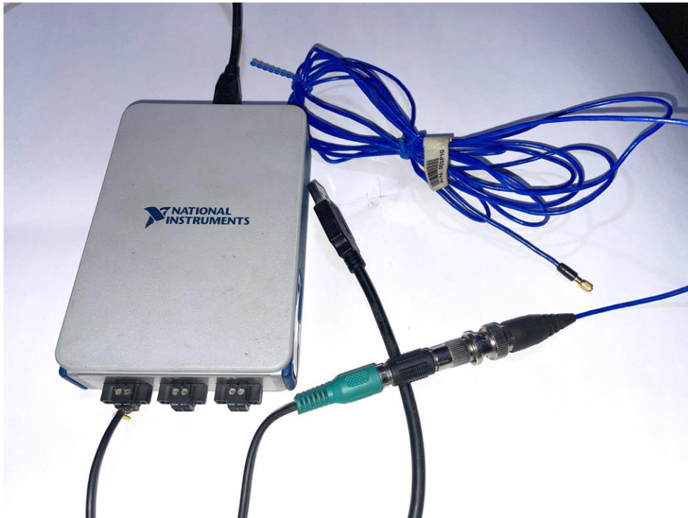
Figure 9.3. NI DAQ system connected with BNC cable
