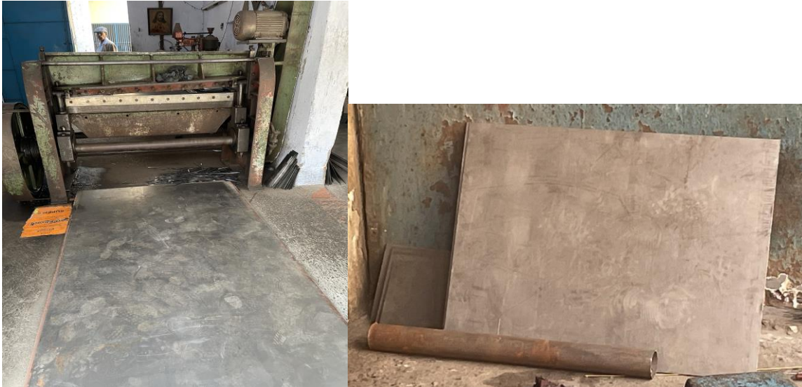
Figure 6.10. (a) Mild steel sheet with the sheet cutting machine, (b) cutted rectangular sheet for muffler construction.
