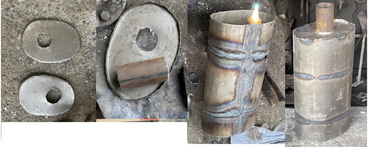
Figure 7.20. Baffles with tubes and muffer after welding all the components
