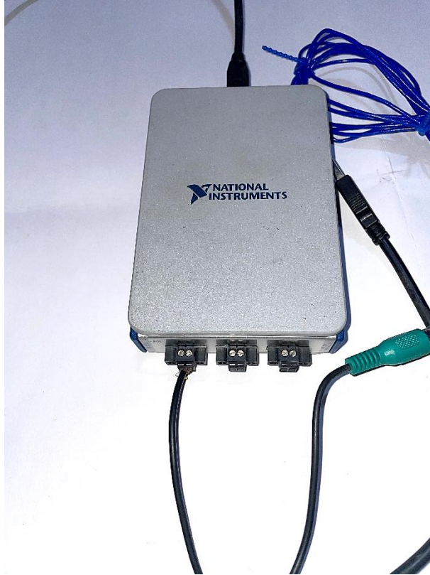
Figure 9.2. Three channel NI Data acquisition system
