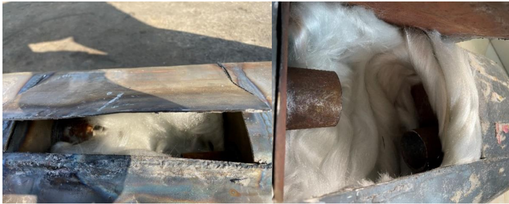
Figure 8.13 Implementing the sound absorption material inside the muffler
