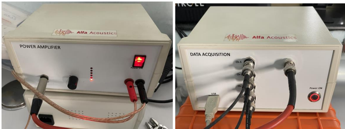
Figure 6.14. (a) Alfaacoustics Power Amplifier, (b) Alfaacoustics Four-channel Data Acquisition System
