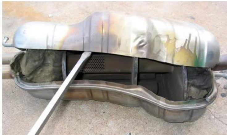
Figure 1.8. Hybrid muffler (Source: Silex Exhaust Silencers, Inc.)
