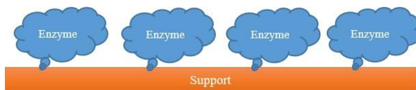
Figure 2.7 Adsorption (enzyme immobilization) technique in which the enzyme is adsorbed by the exterior surface of the matrix or support.
