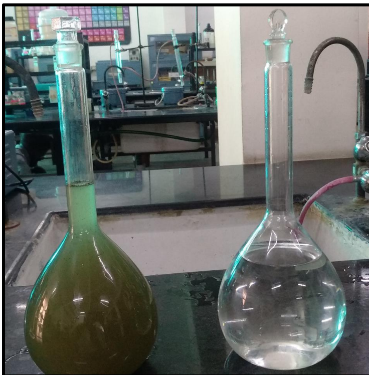
Figure 3.3. A stock solution of weed extract attained after aggregation with 0.5M HCl ( left ), Beaker containing 0.5M HCl solution ( right ).
