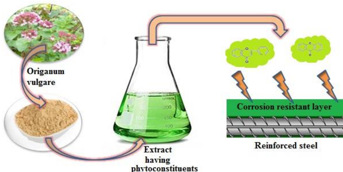
Figure 1.4. Plant ( Origanum vulgare ) extract being used as a corrosion inhibitor for reinforced steel which develops a layer resistant to corrosion. 47
