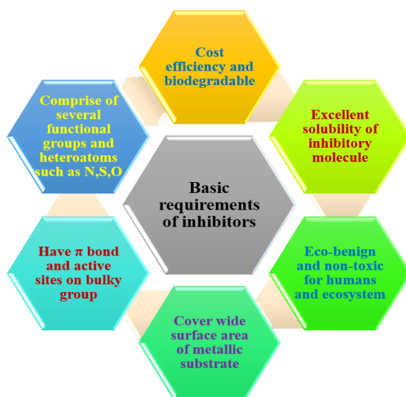
Figure 1.5. Diagram outlining the crucial factors that must be met for compounds to be considered as suitable green corrosion inhibitors for preventing metal corrosion.
