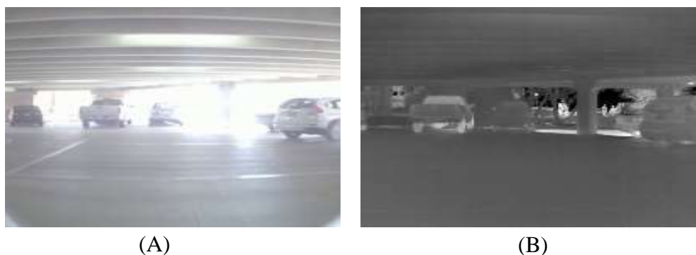
Figure 3.6: Sunlight-affected images from the visible camera (A) and Thermal Camera (B) from FLIR Dataset [221]
