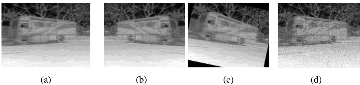
Figure 3.9: Augmented Images (a) original (b) flipping (horizontal) (c) rotation (d) gaussian noise [221]
