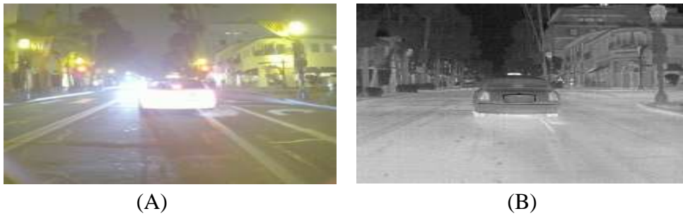
Figure 3.8: Nighttime image from the visible camera (A) and Thermal Camera (B) from FLIR Dataset [221]
