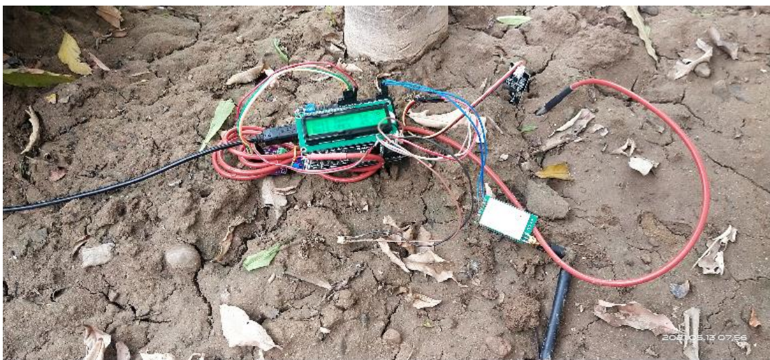
Figure 3.11 Wireless soil sensor node
