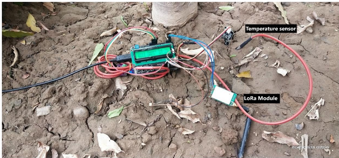
Figure 4.6 Soil sensor node deployed in farmland
