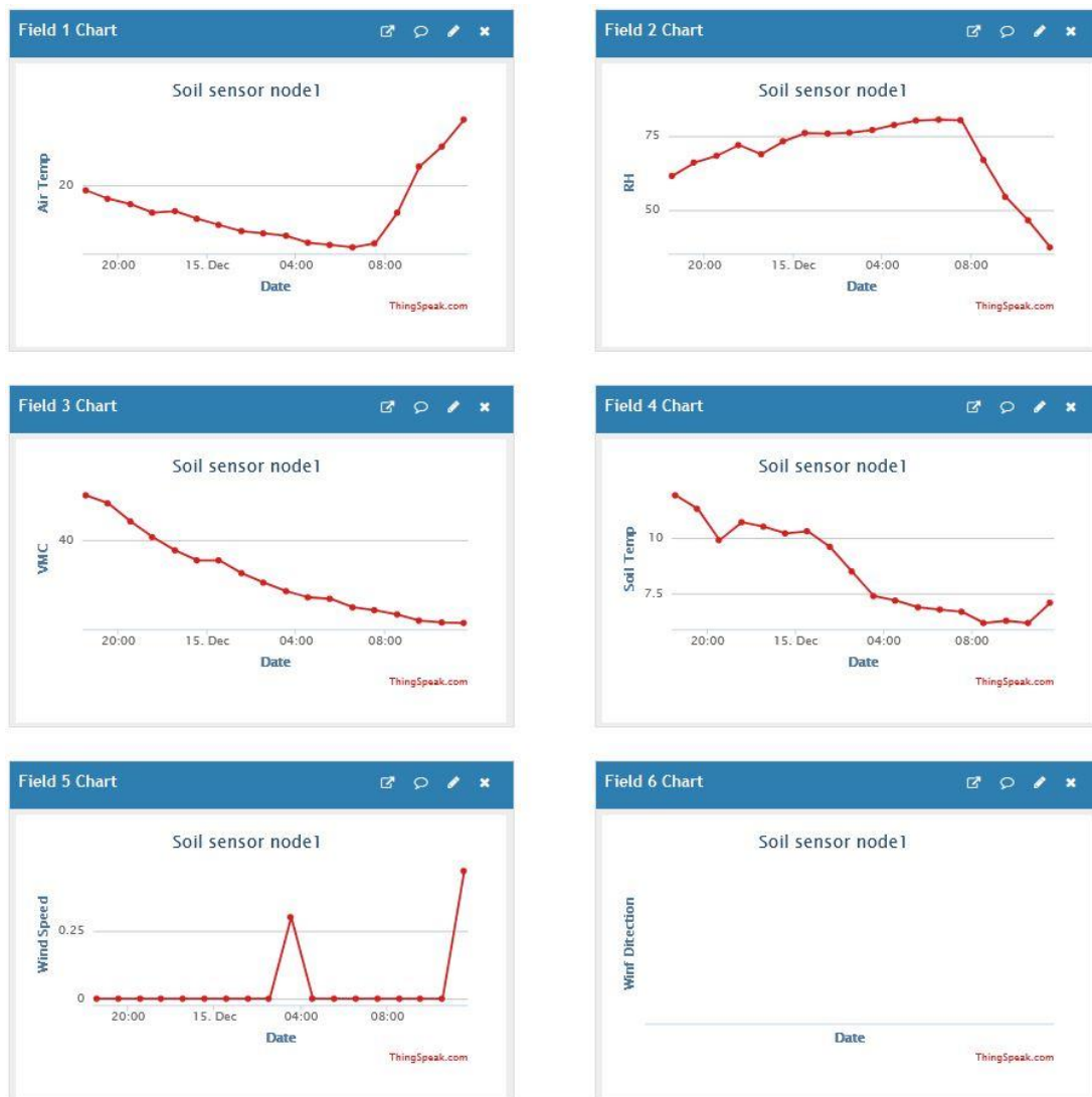
Figure 4.13 Thingspeak data visualization for soil sensor node 1
