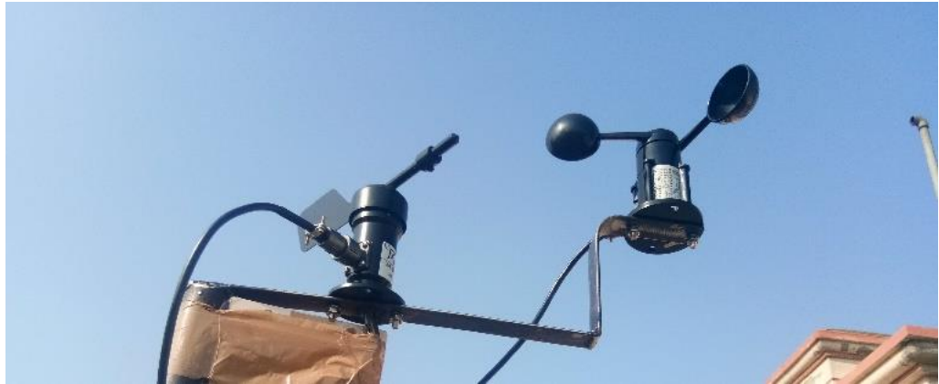
Figure 3.13 Wind direction and wind speed sensor
