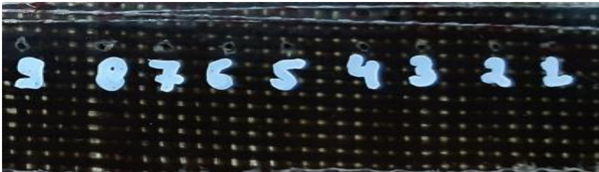
Fig. 5.2: Image of top side of hybrid KBFRP composite after laser drilling
