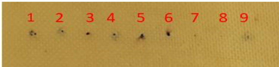
Fig. 4.4: Image of bottom side of KFRP composite after laser drilling
