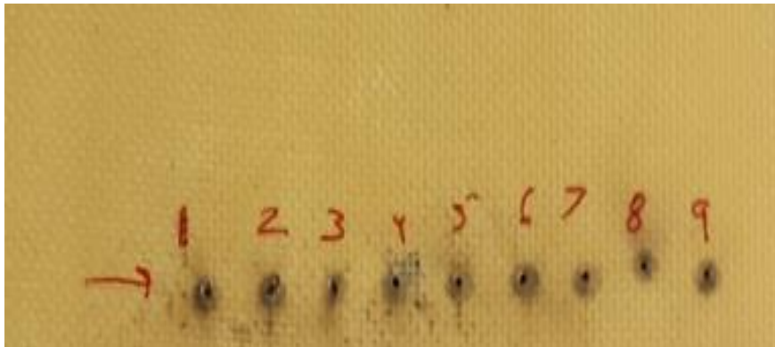
Fig. 4.2: Top side image of KFRP composite after laser drilling
