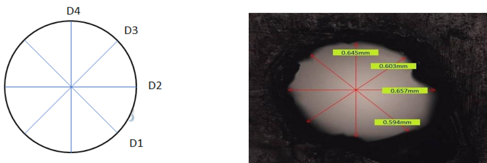
Fig.5.6: (a) Schematic measurement of hole diameter (b) Actual measurement
