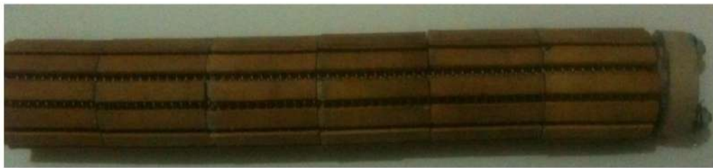
Figure 3.23 Photograph of Manufactured Gas Heater
