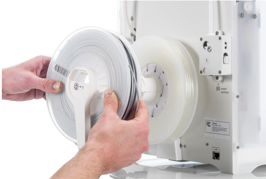
Figure 3.5 Feed System for Model and Support Material
