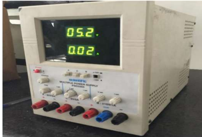
Figure 3.12 Direct Current Rectifier
