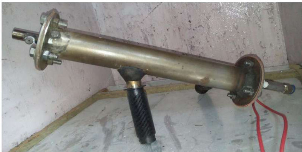
Figure 3.24 Photograph of Gun Casing and Mountings
