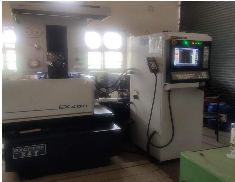
Fig.3.2 EDM M/C used for cutting of samples
