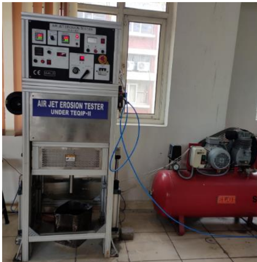
Fig.3.5(a) High temperature air jet erosion test rig set-up used for Experimentation.
