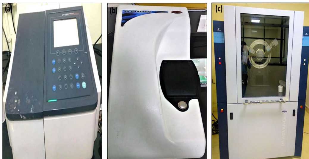
Fig. 3.3 (a) UV-vis spectrophotometer (b) zeta potential and particles size analyser (c) X-ray Diffractometer
