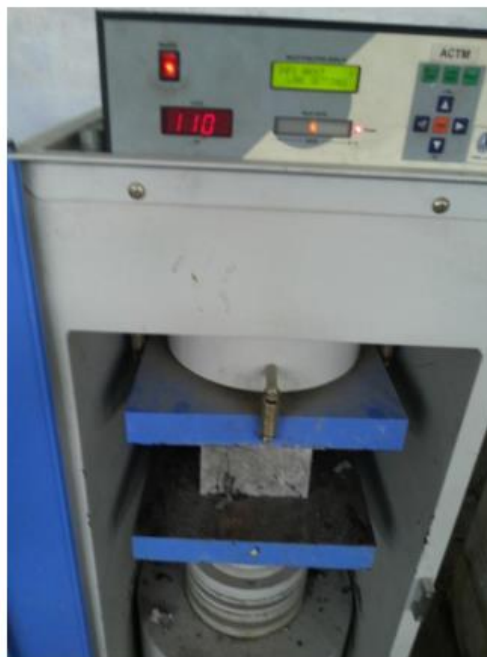
Figure 3-8 Compression test setup
