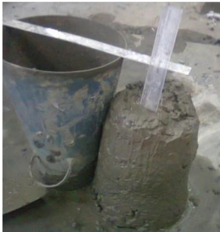
Figure 3-7 Setup of slump test
