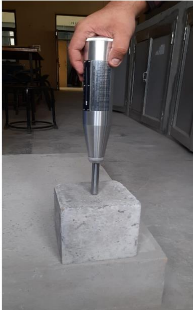
Figure 3-13 Rebound hammer testing device
