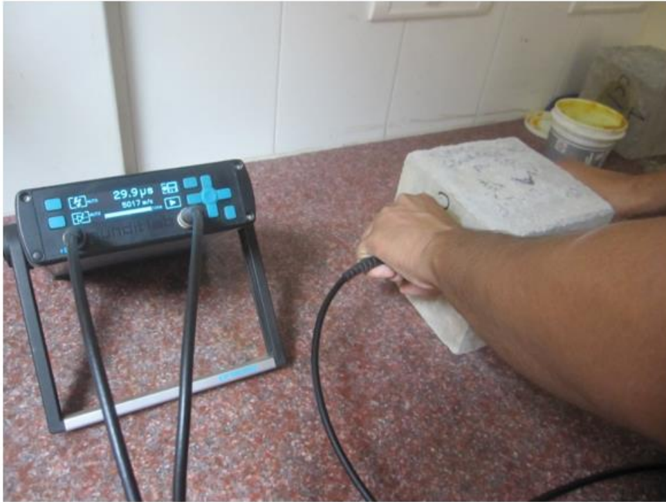
Figure 3-12 Experimental set up for measuring pulse velocity through concrete
