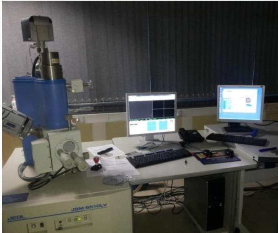
Figure 3-17 Experimental set up for Scanning Electron Micrograph
