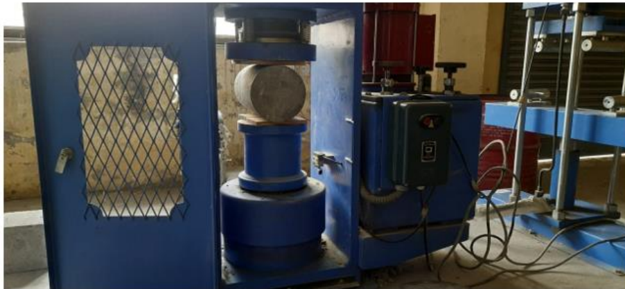
Figure 3-9 Splitting tensile strength setup
