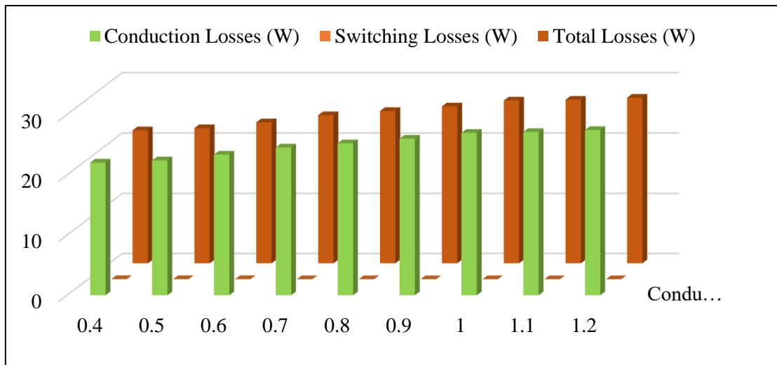
Figure 4.20 Power losses Vs modulation index using precise Simulink models
