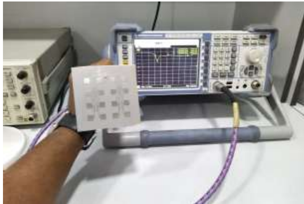
Figure 6.4(a): Testing of the antenna for measurement of return loss
