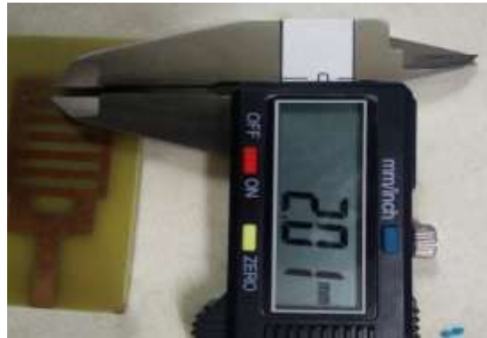
Figure 5.5. Width of the inner rectangle slot depicts 2.01 mm
