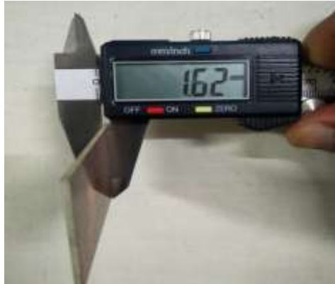
Figure 5.4. Width of the substrate height depicts 1.62 mm
