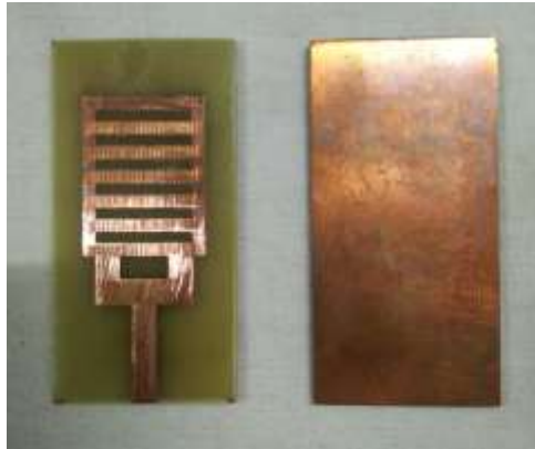
Figure 5.10. Fabrication of proposed antenna by using printed circuit board material “duriod”
