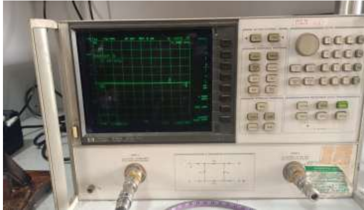
Figure A. 1VNA Equipment used for proposed antenna Return loss and VSWR measurement
