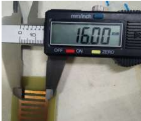
Figure 5.6. Width of the inner rectangular slot depicts 16mm
