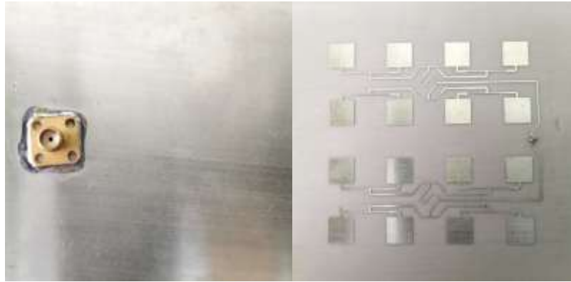
Figure 6.3: Front to back side image for fabricated antenna
