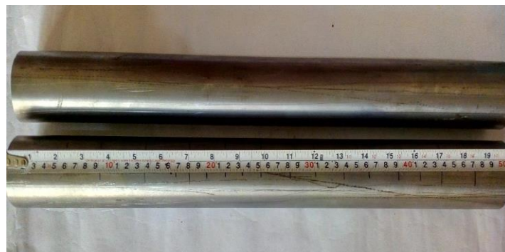
Figure 5.3: Titanium Gr 2 workpiece rod of diameter 50 mm and length 510 mm.
