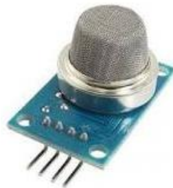
Figure 3.31 Smoke detection sensors
