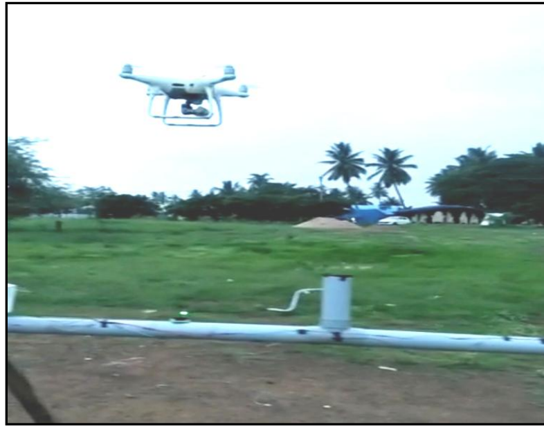
Figure 7.5 Drone inspecting pipeline
