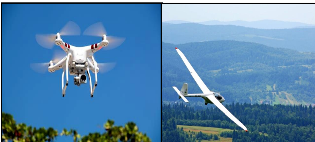
Figure 1.11 UAS systems. a) Quadrotor (b) Fixed-wing [48]
