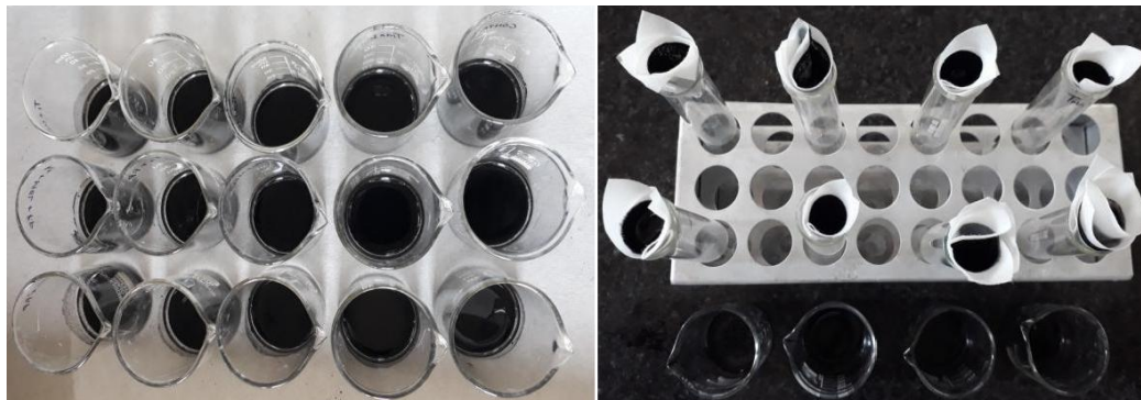
Figure 5.14: Addition of activated charcoal to amalgam and filtration process using Whatman filter paper #1.
