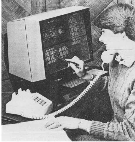
Figure 7.12: A Microfiche Reader: The 3M Model 148. (Courtesy of 3M Micrographic Products Division)
