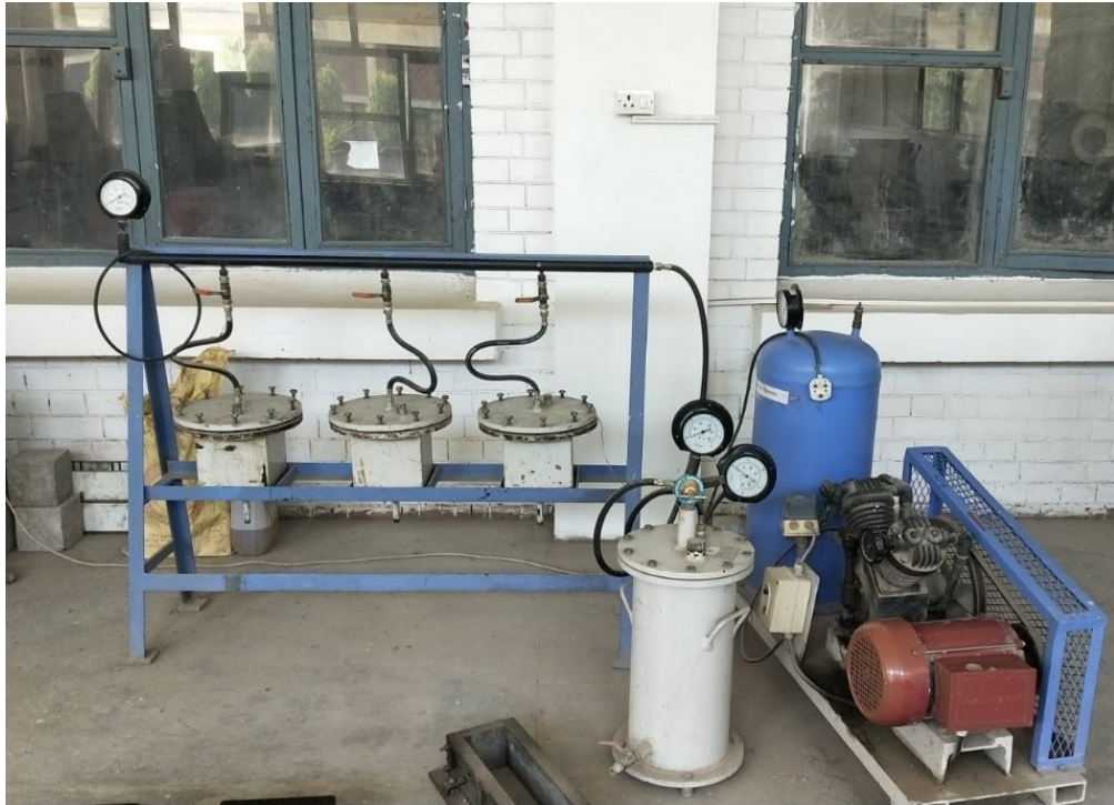
Figure 4.17: Permeability test of concrete cubes
