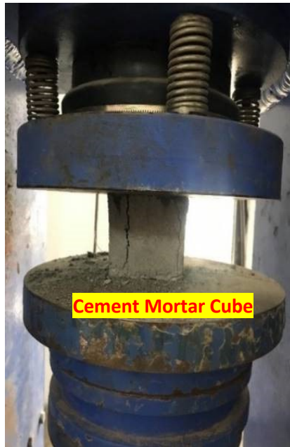
Figure 4.5: Compressive strength Test of Cement Mortar Cube of Size 70.6 x 70.6 x 70.6 mm 3
