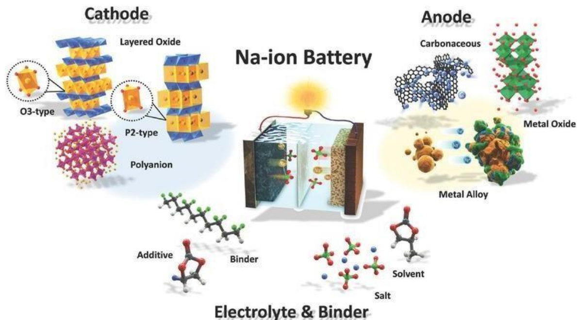
Figure 1.8 Various components of a Na-ion battery system
