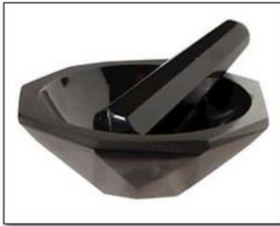
Figure 3.11: The agate mortar and pestle used for fine grinding of powders.
