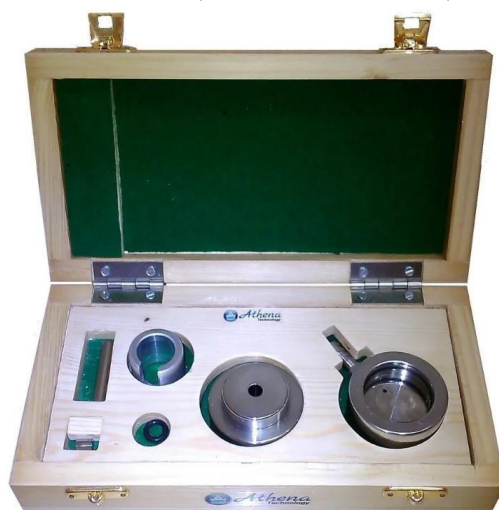
Figure 3.12: Cold Press Die-set of 12 mm diameter.
