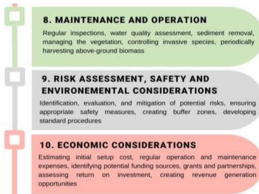
Fig.6.1 Key considerations during various stages of designing constructed wetland treatment systems
