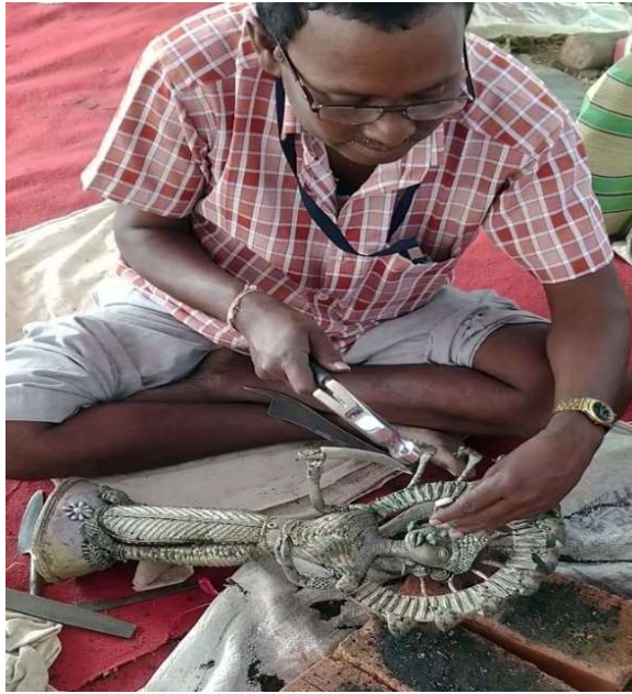
Figure 3.2.23 Nails are removed from the cast with chisel Figure
