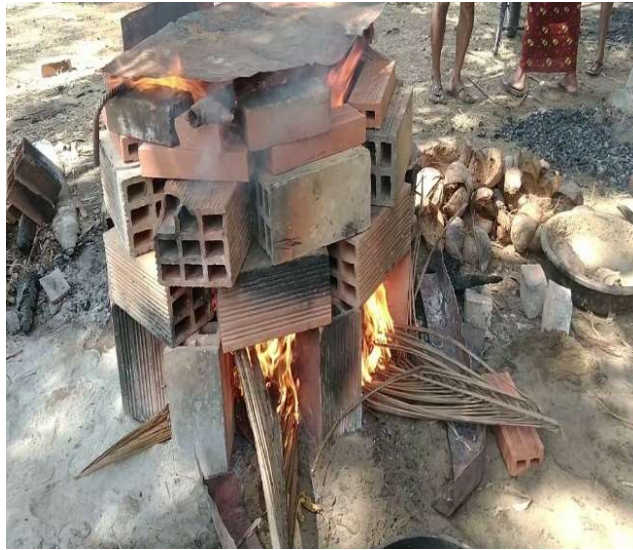
Figure 3.3.12 Final firing of moulds for the complete De-waxing.
