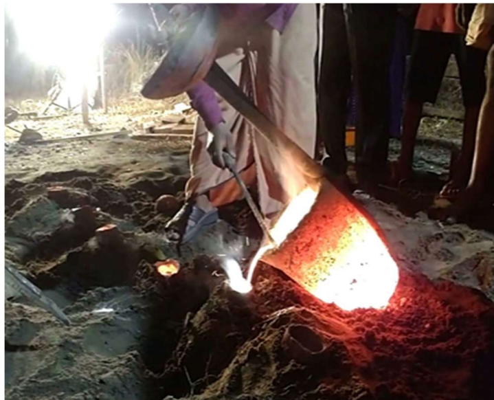
Figure 3.3.14 Pouring of molten metal into the moulds, buried in the ground pit with mould pouring mouth facing out upwards.
