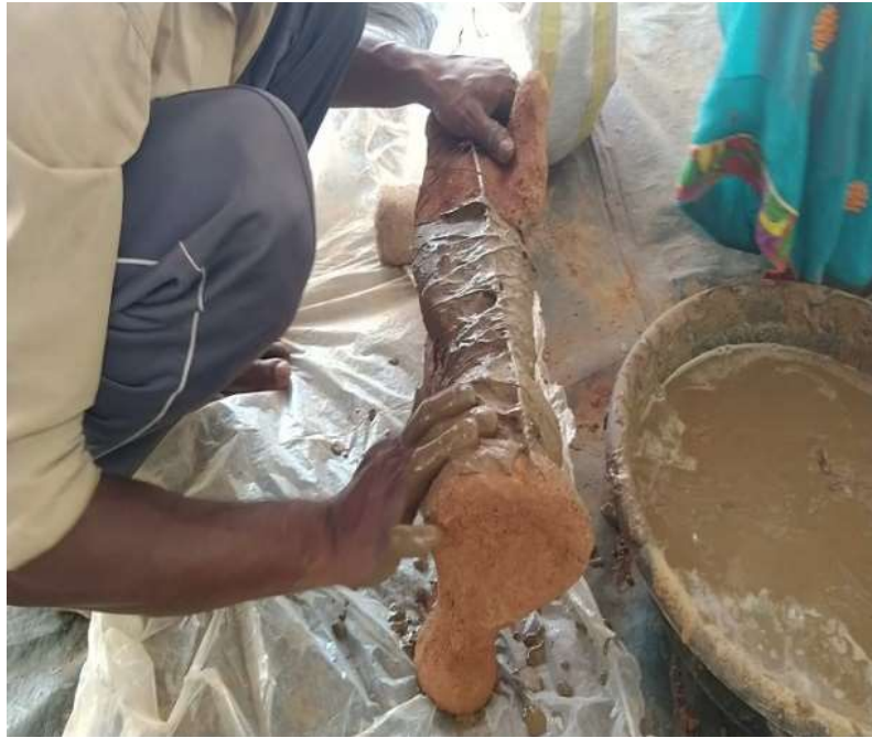
Figure 3.2.13 Last layer of clay is added on the mould
