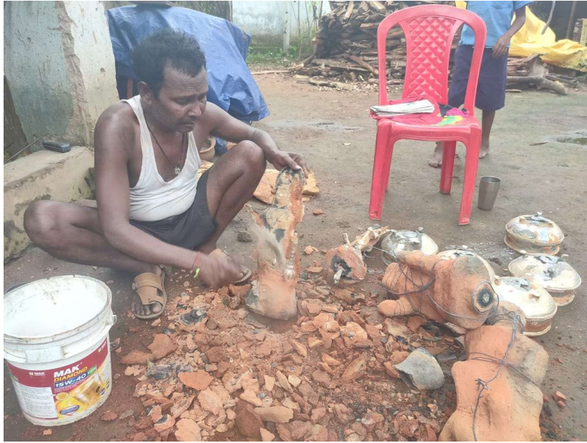
Figure 4.6 Tribal sculptor Banno Ram removing mould layer after casting
