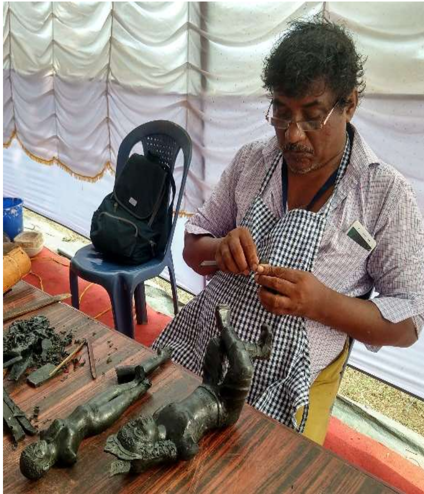
Figure 3.3.3 Wax modelling using a knife and scraper.
