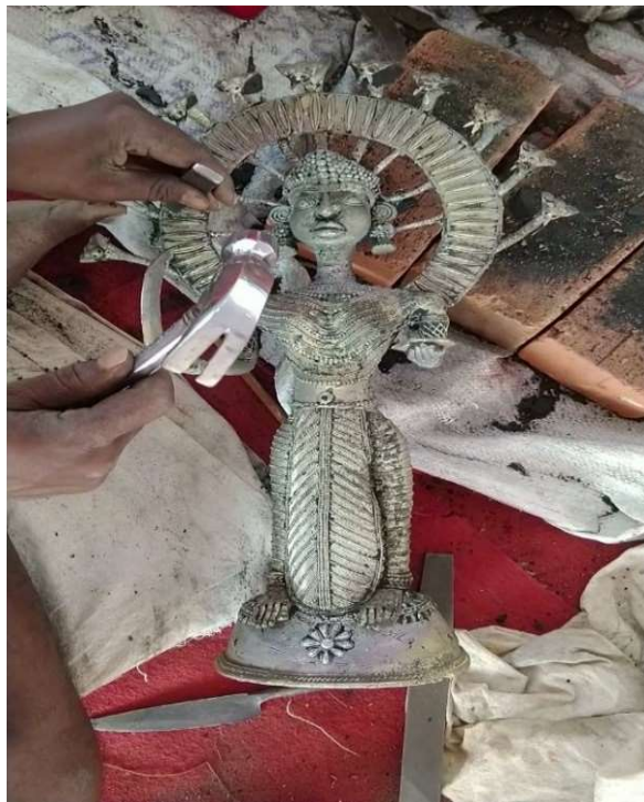
Figure 3.2.24 Unwanted metal flashes are chiselled carefully.
