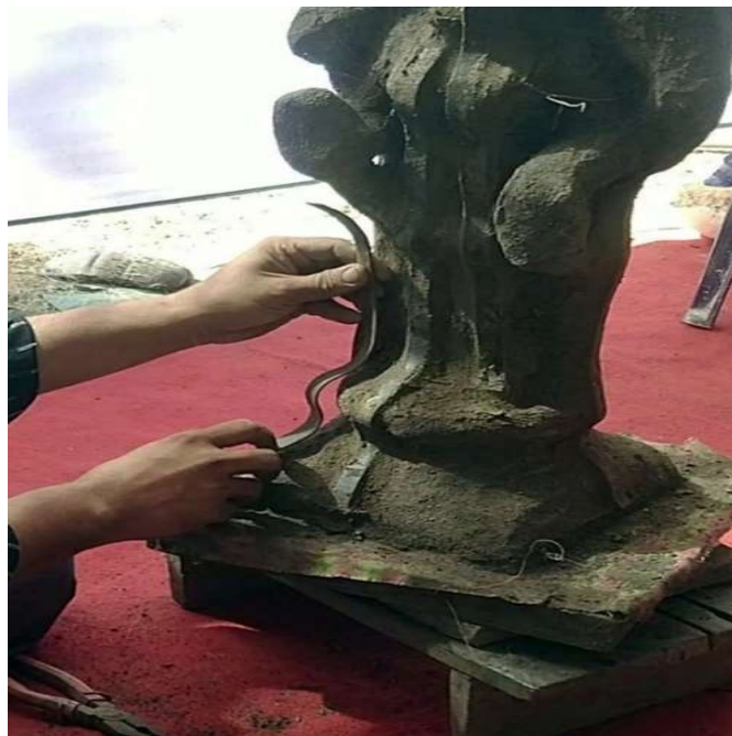
Figure 3.3.8 Iron strips are added to strengthen the mould.
