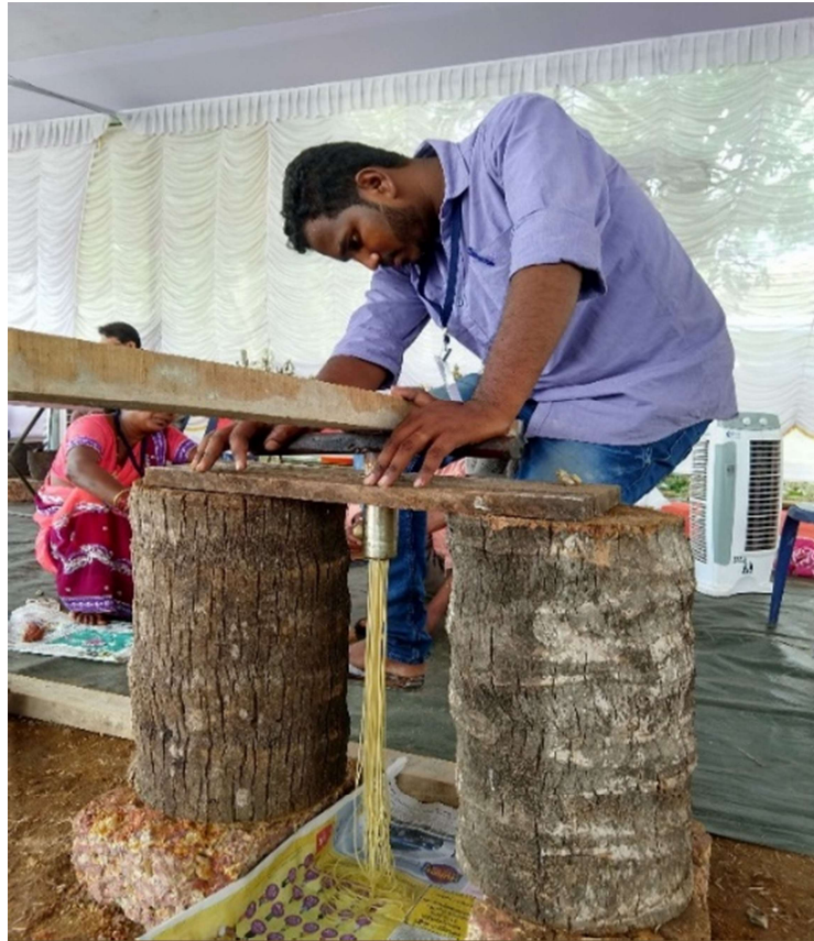
Figure 3.2.2 Creating Wax strings of soft bee's wax from a press mould.
