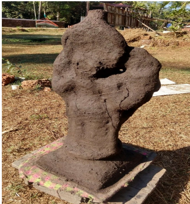
Figure 3.3.9 Moulds is place under the sun for initial dry process.
