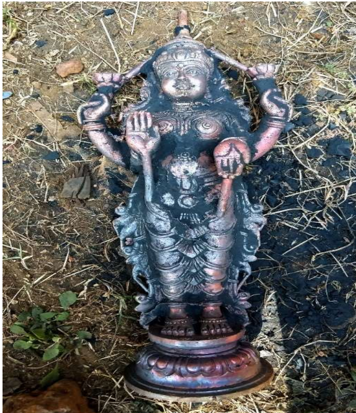
Figure 3.3.15 Mould is removed from the cast.
