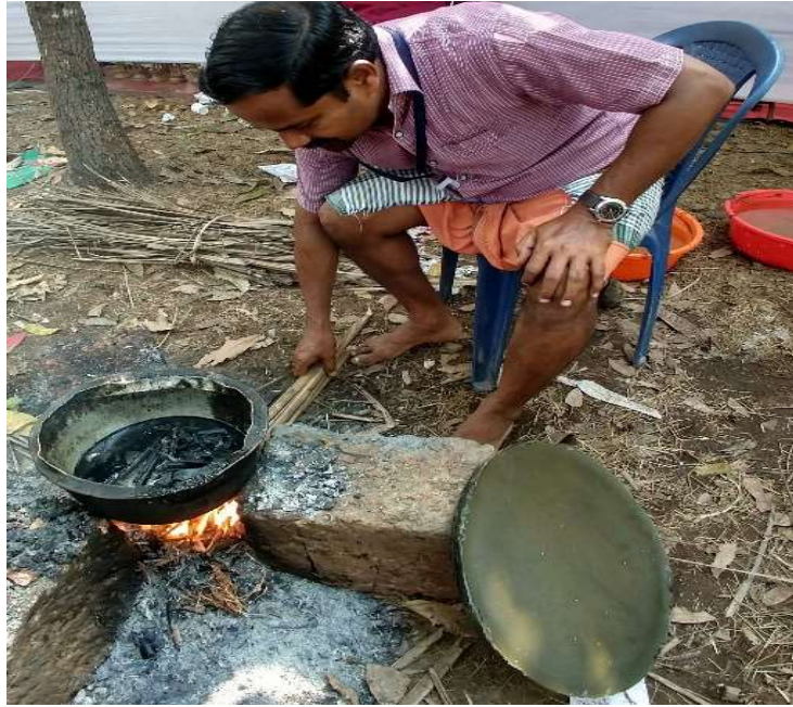
Figure 3.3.1 Melting wax with pine tree gum and black oxide.
