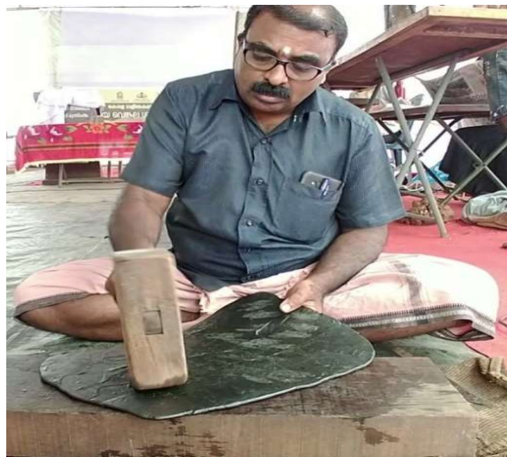
Figure 3.3.2 Creating Wax sheet by beating wax with wooden mallet.
