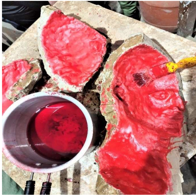
Figure 3.4.1 Wax application on plaster mould
