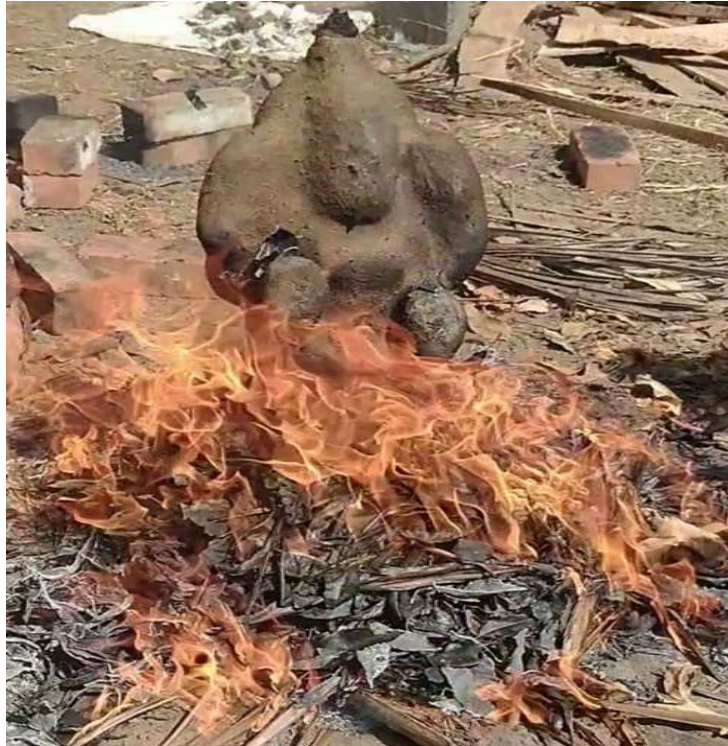
Figure 3.3.10 Initial de-waxing process by open firing
