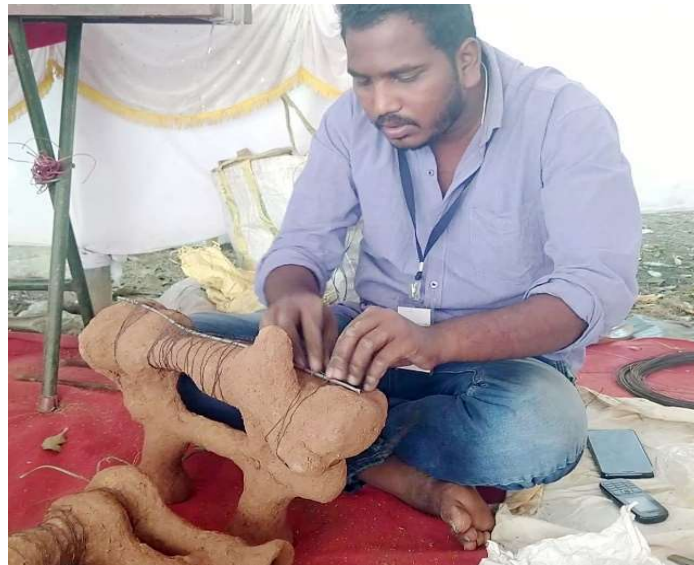
Figure 3.2.12 Galvanised wire and binding wire are used to reinforce the mould
