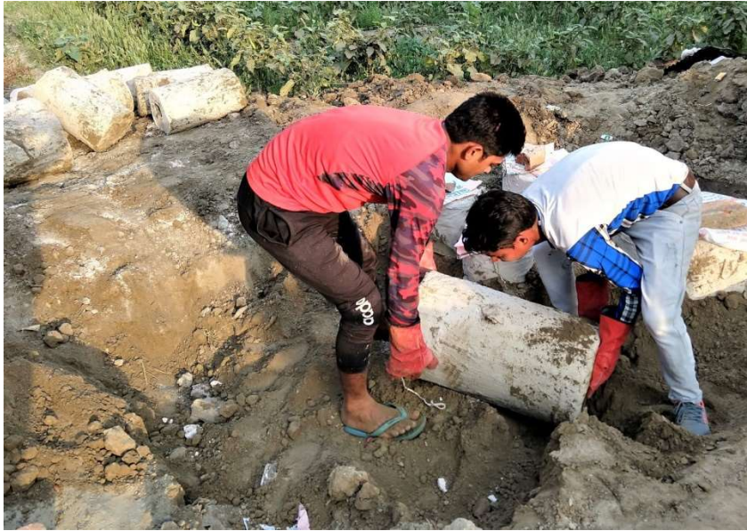
Figure 3.4.12 Investment moulds are taken out from the pit after solidification on metal
