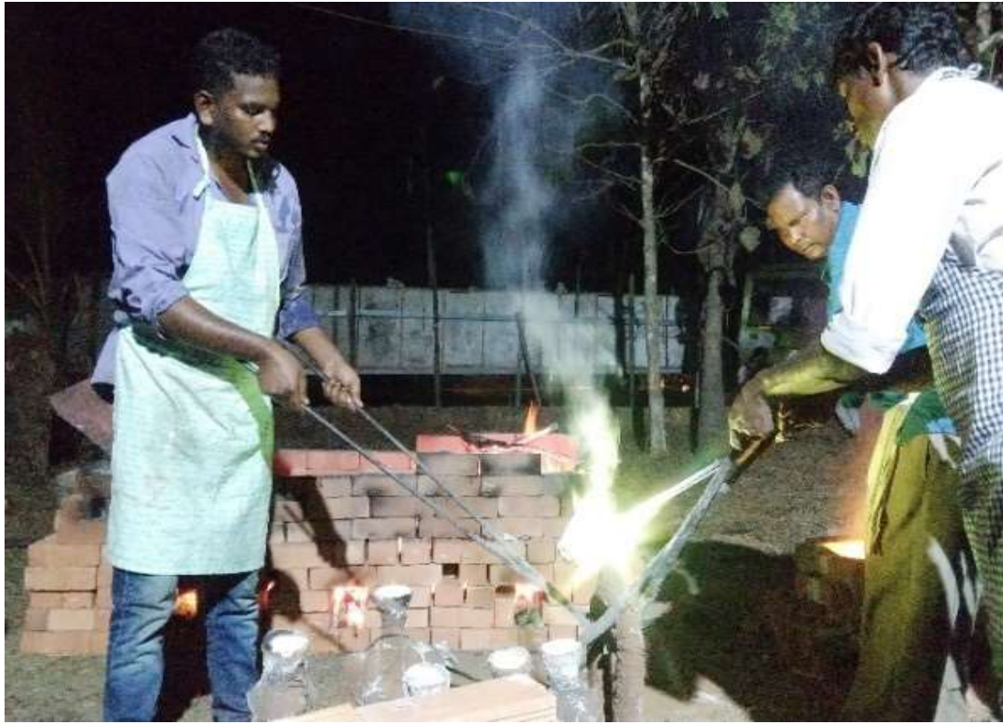
Figure 3.2.20 Pouring of molten metal into the moulds
