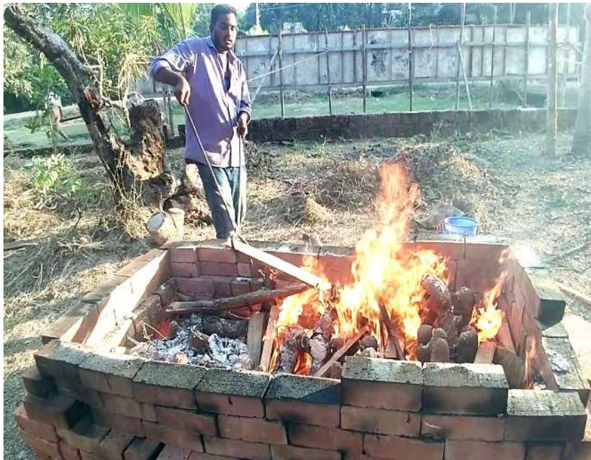
Figure 3.2.18 Iron tongs are used to add woods gently around the moulds
