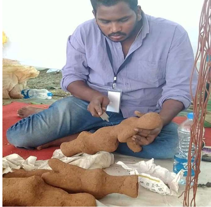
Figure 3.2.11 Iron nails are added as core pins.
