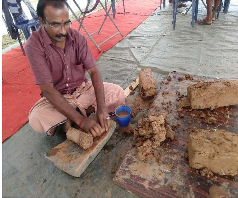
Figure 3.3.5 Preparation of clay for mould making process.
