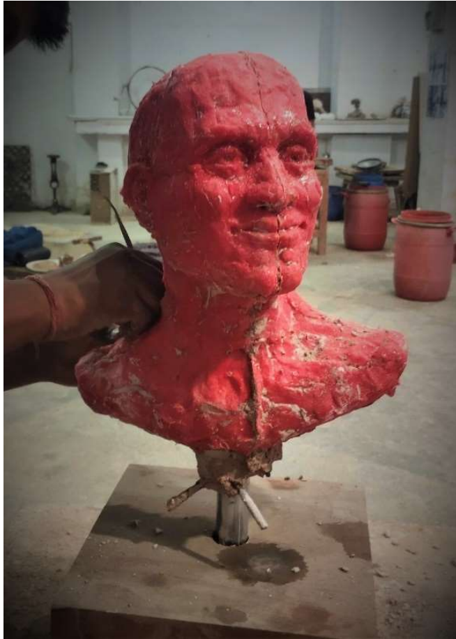
Figure 3.4.2 Finishing wax model with steel tool
