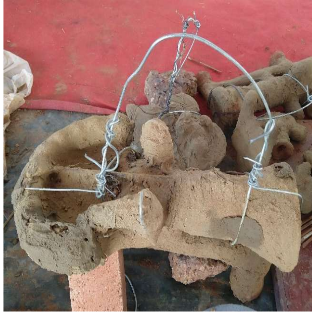
Figure 3.2.15 Handel is created with galvanised wire on large size moulds
