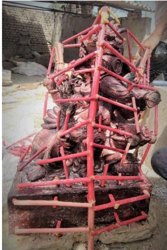
Figure 3.4.8 Wax runners attached to finished wax model
