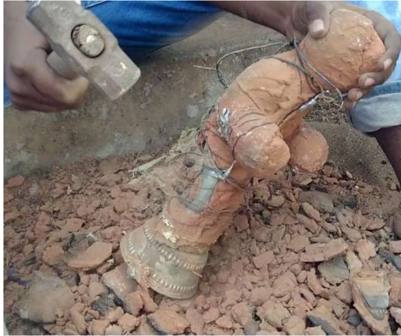
Figure 3.2.21 The mould is removed from the cast with a hammer.
