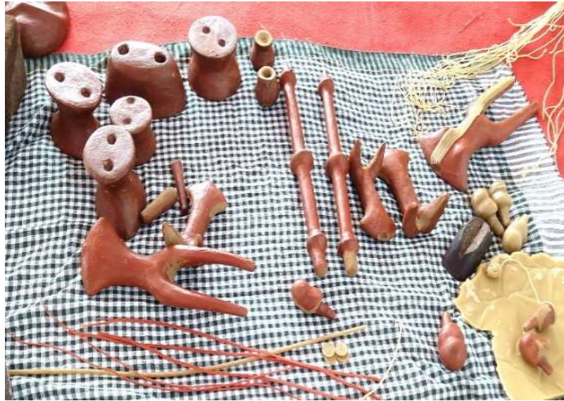
Figure 3.2.4 Wax layer is applied on sundried clay core body.
