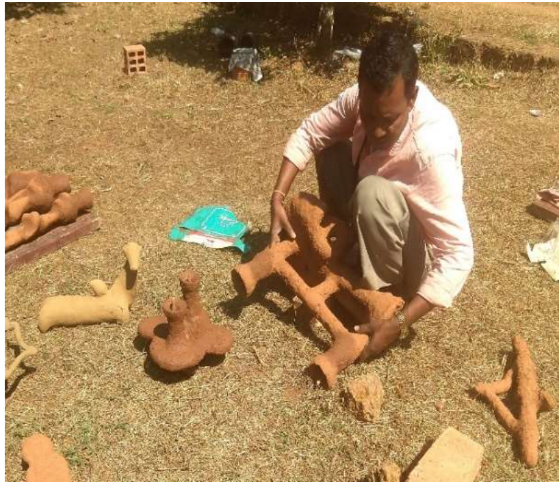
Figure 3.2.14 Moulds is place under the sun for initial dry process
