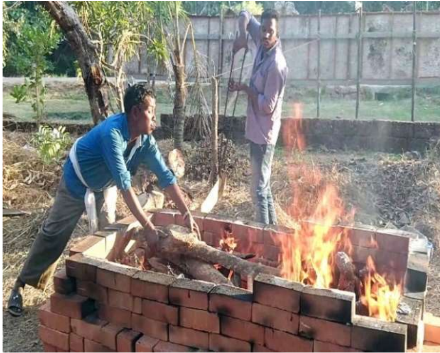
Figure 3.2.17 Dewaxing process of moulds in local kiln
