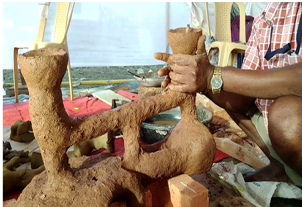
Figure 3.2.10 Clay funnel is attached with wax runner on the mould
