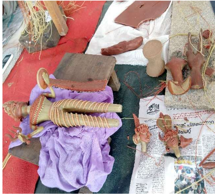
Figure 3.2.6 The wax model is kept on piece of cloth, to assemble the parts
