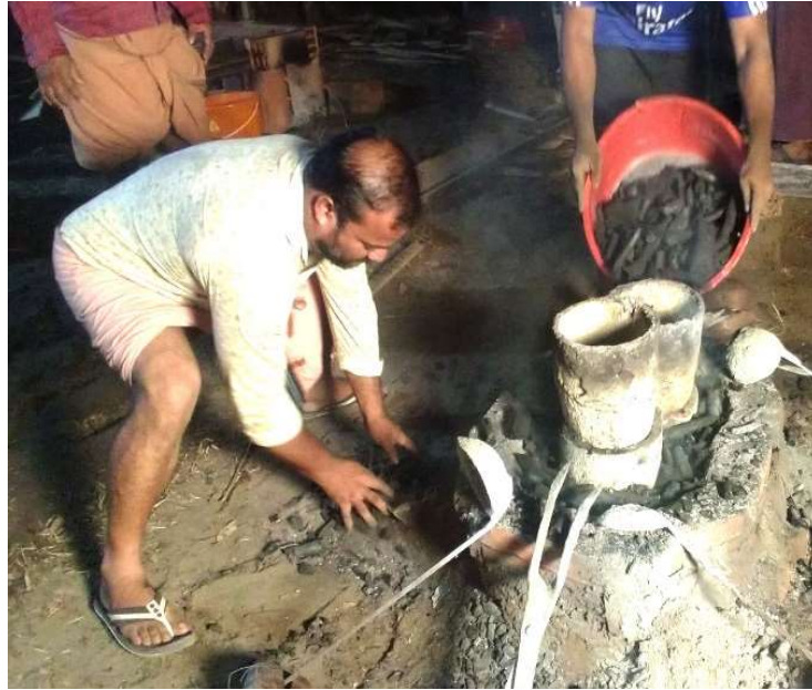
Figure 3.3.13 Traditional furnace with coal firing for melting the metal.
