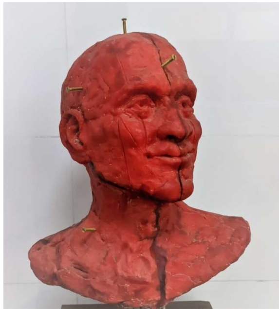
Figure 3.4.7 Wax model with core pins
