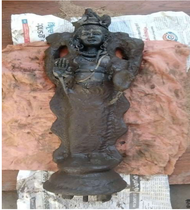
Figure 3.3.7 While mould making process, wax model is kept on piece of cloth.
