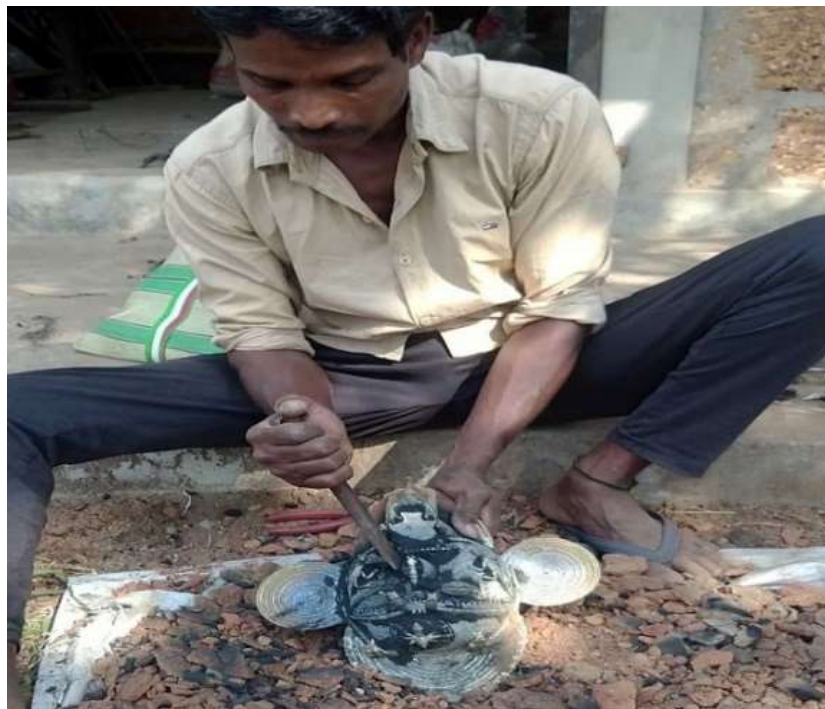
Figure 3.2.22 Chisels are used to remove the mould remains.
