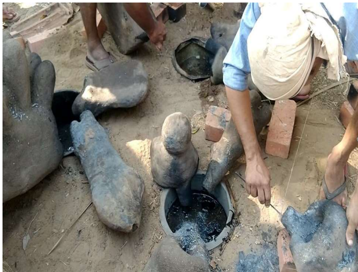
Figure 3.3.11 Mould are place on a vessel to collect the wax.
