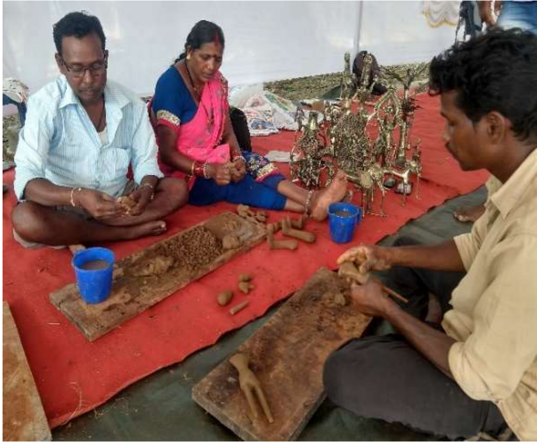
Figure 3.2.3 Creating core body with clay.
