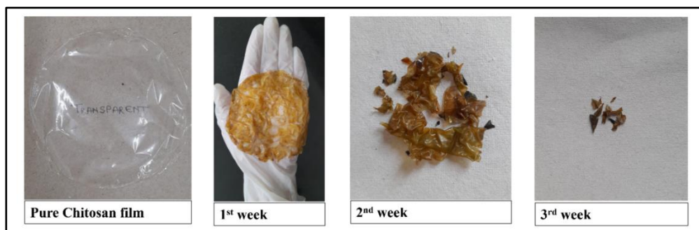
Figure 4.29: Fastest degradation process of pure chitosan film
