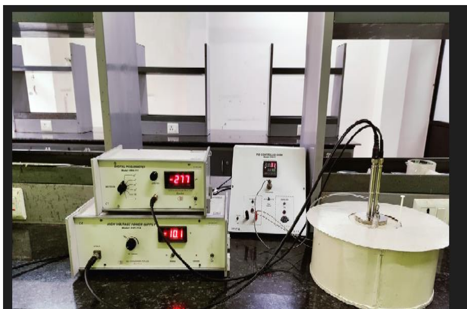
Figure 3.24 Experimental set-up of thin film gas sensor for measuring response toward H 2 S gas.
