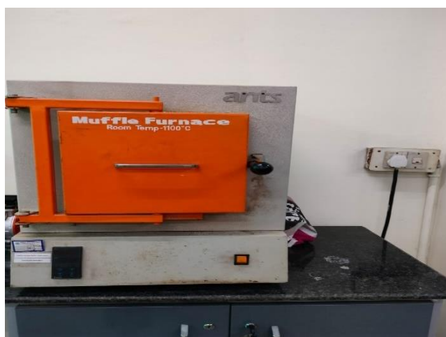
Figure 3.3 The muffle furnace used for annealing of thin films.
