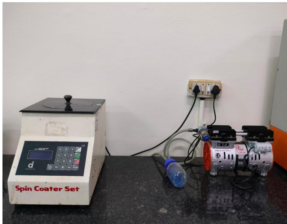
Figure 3.2 The above figure shows the spin coater for fabrication of thin films.
