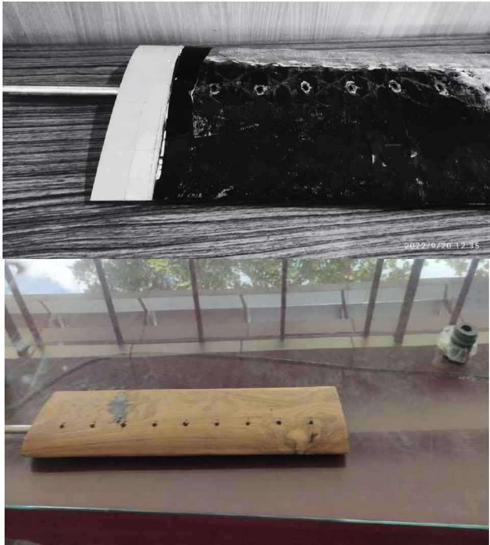
Figure 516 : Designing wing model with vents by using 3d printing and teakwood
