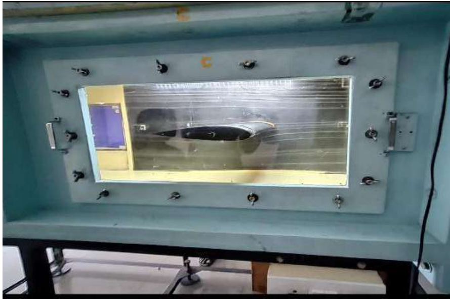
Figure 519 : wind tunnel section 600*600mm testing of airfoil
