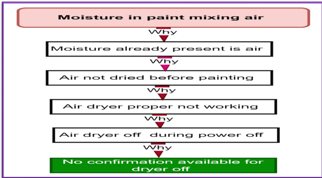
Figure 6.32— Moisture in Paint Air Mixture
