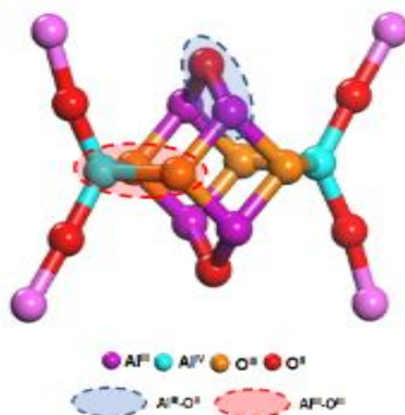
Figure 21: The structure of 20 atom clusters of bulk \text{Al}_2\text{O}_3 (110) surface with \text{Al}^{\text{III}}\text{-O}^{\text{II}} and \text{Al}^{\text{III}}\text{-O}^{\text{III}} site pairs adjacent to each other {Obtained using Pople 6-311G(d)/MO6-2x}
