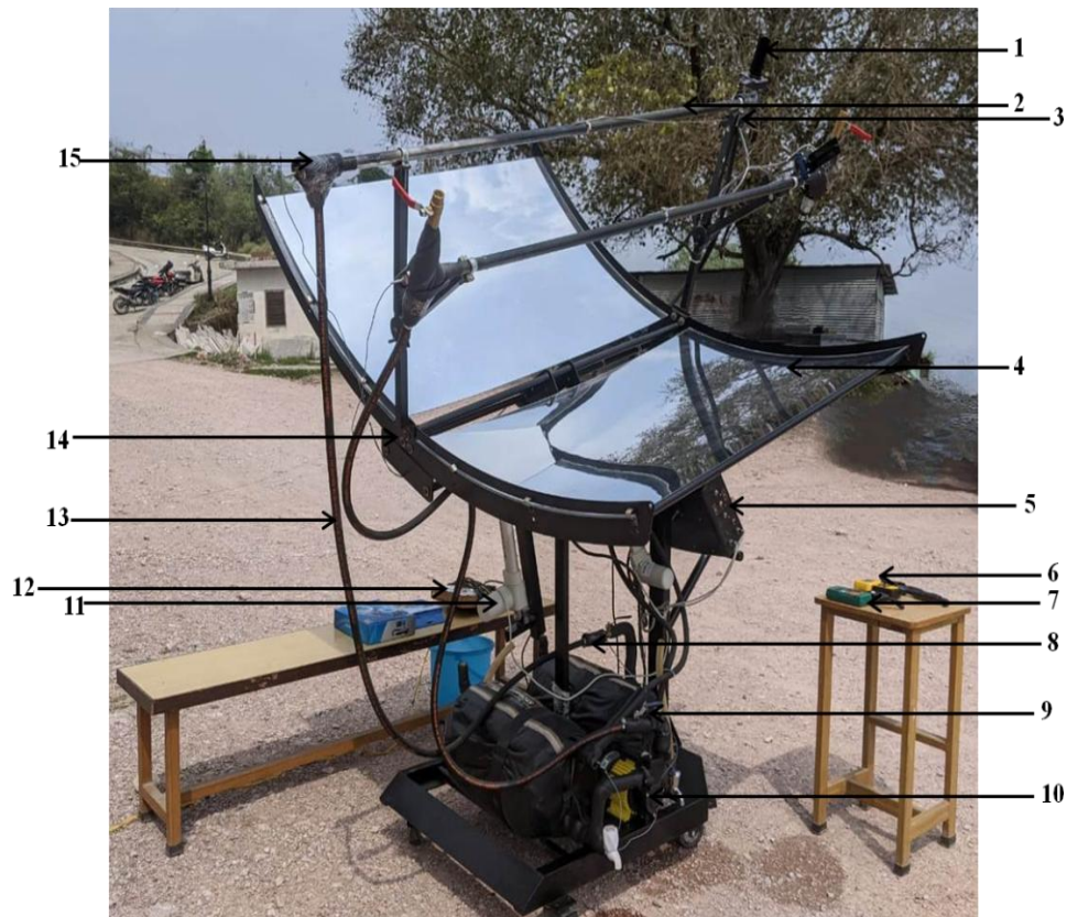
(1) Light Dependent Resistor, (2) Stainless Steel Receiver Pipe, (3) Water Inlet, (4) Acrylic Mirror, (5) Control and Display Unit, (6) Digital Anemometer, (7) Solar Flux Meter, (8) Water Flow Sensor, (9) Water Storage Tank, (10) Pump, (11) Sun Tracking Actuator, (12) Power Supply, (13) Hydraulic Hose Pipes, (14) Parabolic Trough, (15) Water Outlet
