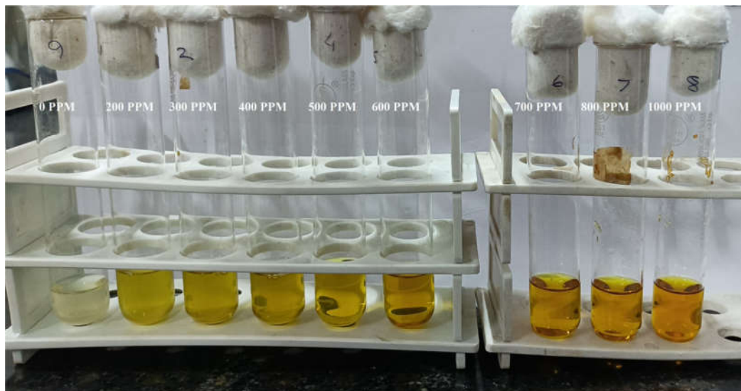
Figure 6.5: Growth of the isolate in increasing concentration of Cr(VI) supplemented nutrient broth for MIC determination. Growth can be observed upto 400 ppm
