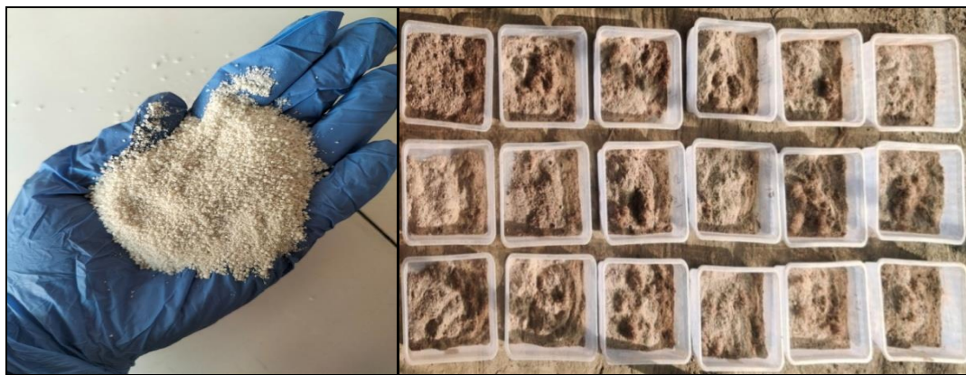
Fig 5.1(a) Polypropylene microplastics used for the experimental study b) The mixture of artificial soil (Kaolinite clay, Sand and Coco peat).
