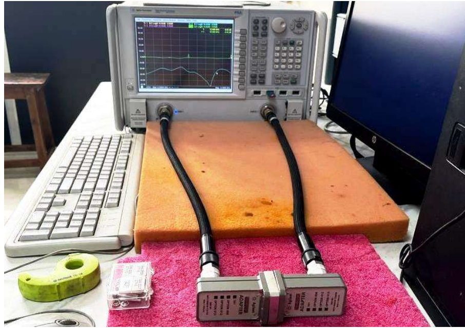
Fig. 3.5 Measurement of parameters using VNA
