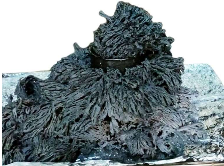
Fig. 3.2 Sample prepared using sol-gel method
