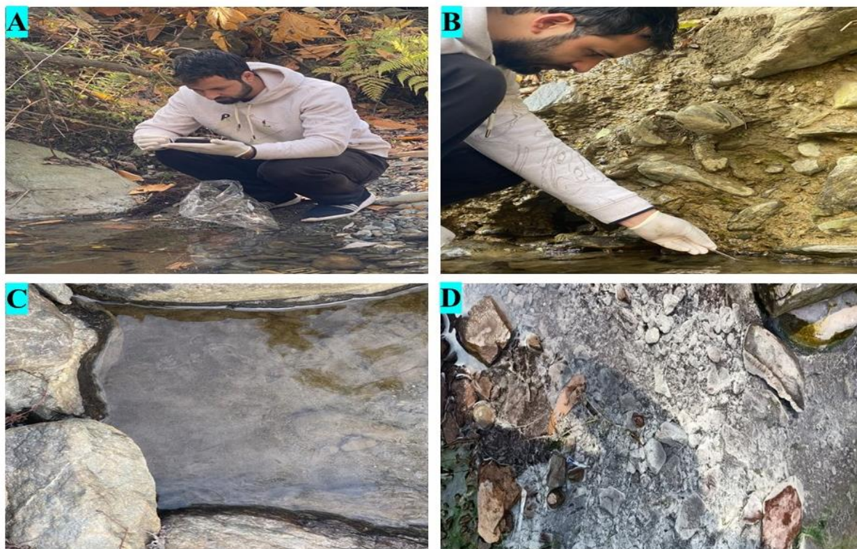
Figure 4.2: RHS sample site (A) Temperature check, (B) Measurement of electrical conductivity, (C) Origin of RHS water, (D) Sulphur deposition on RHS drainage.
