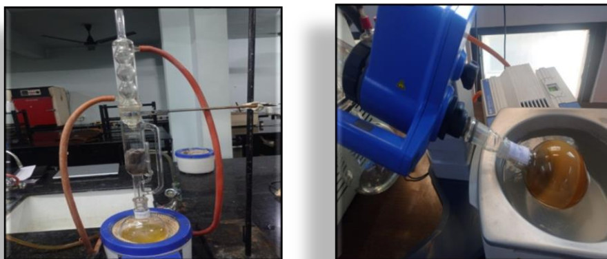
Fig 5.1. Preparation of extract using a Soxhlet apparatus
