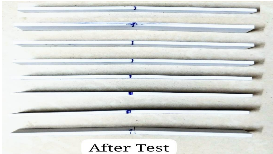
Figure 4.15 Flexural specimens after testing
