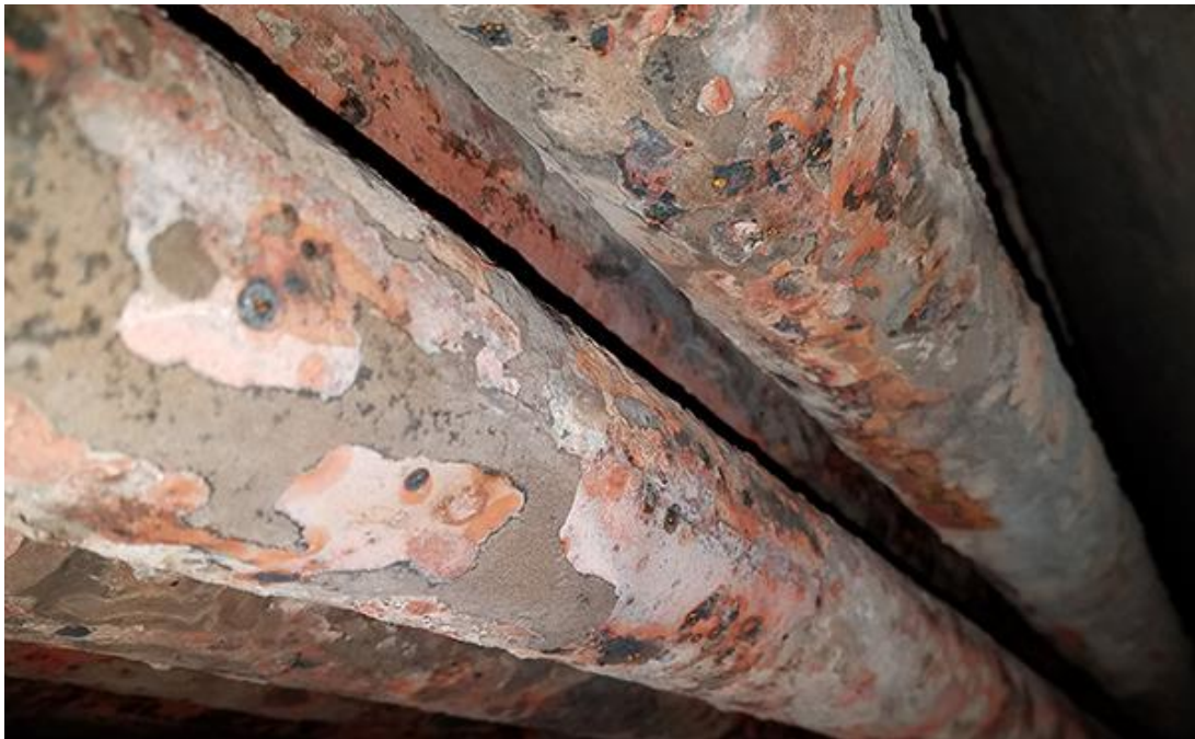
Fig.1.2 Surface corrosion and scale on a boiler shell are depicted ( https://www.watertechusa.com/boiler-blowdown )
