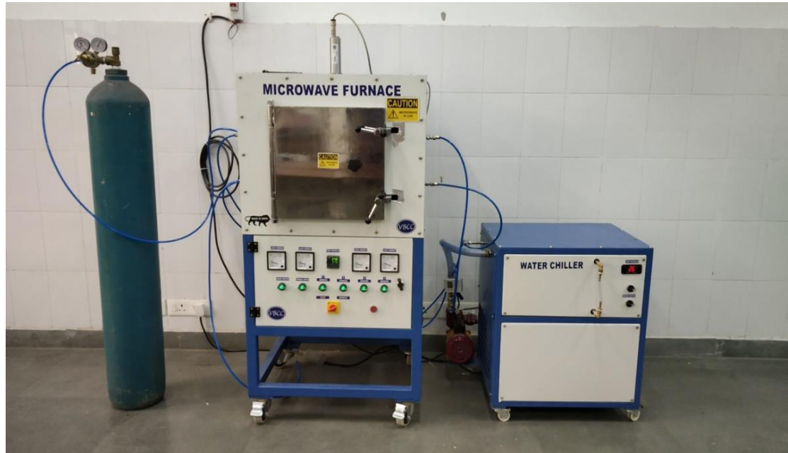
Fig.3.6. Utilization of a microwave furnace to process flame-sprayed coatings post-spray.
