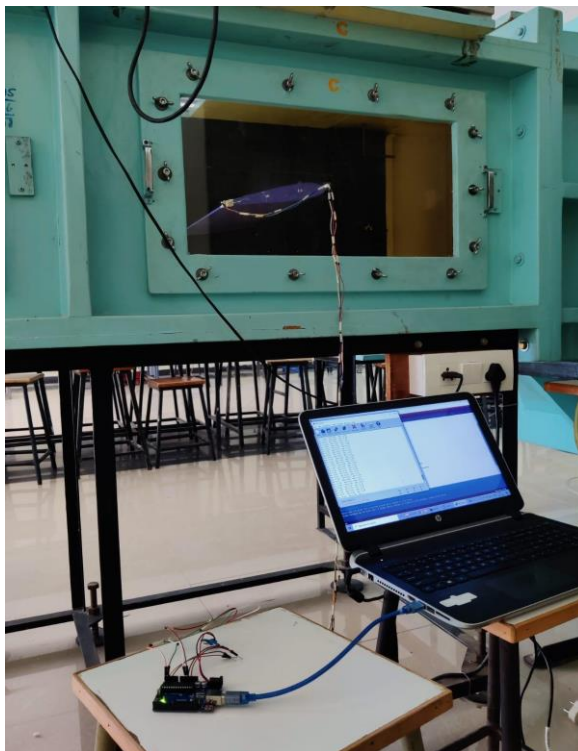
Figure 9. Arduino setup with wing mounted in a wind tunnel.
