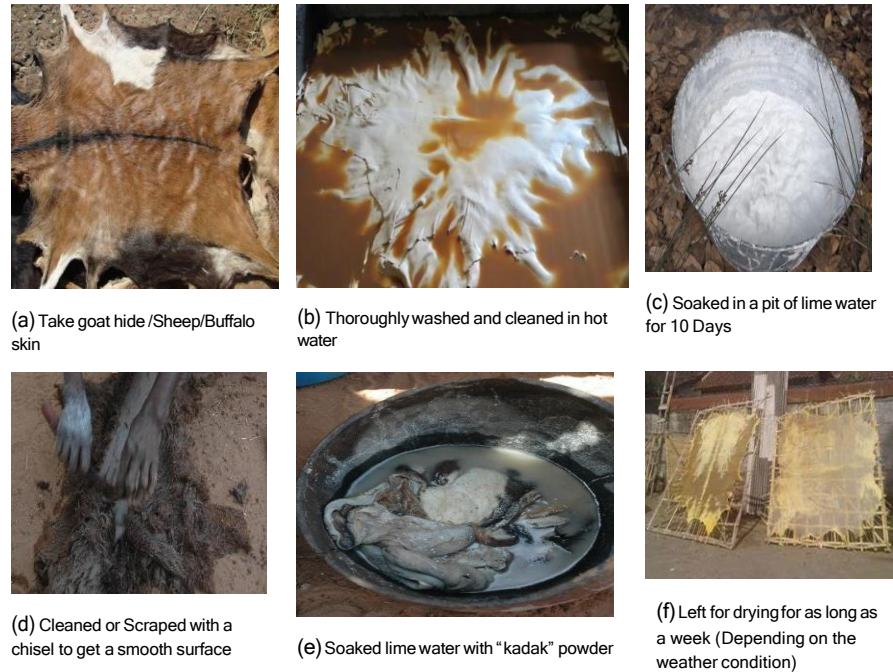
Figure:4.17 (a), (b), (c), (d), (e), &(f)Traditional method of Leather preparation -Step-by-step[Image source: Research scholar]
