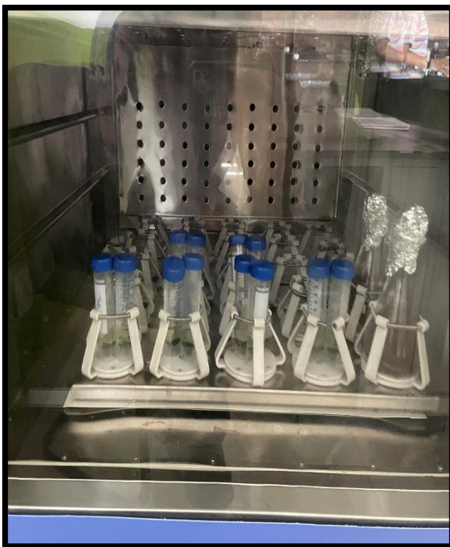
IMG 5: Estimating electrolyte leakage index (using a shaker & EC meter)
