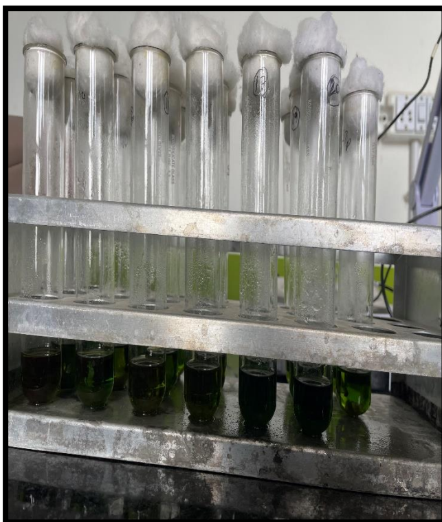
IMG 2: Extracting & estimating chlorophyll in spectrophotometer
