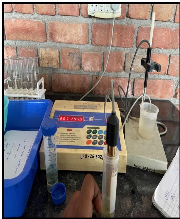
IMG 5: Estimating electrolyte leakage index (using a shaker & EC meter)
