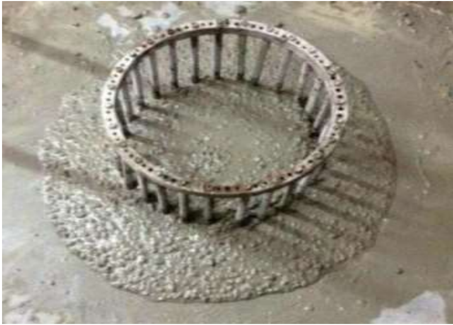
Figure 4.6: J Ring Test
