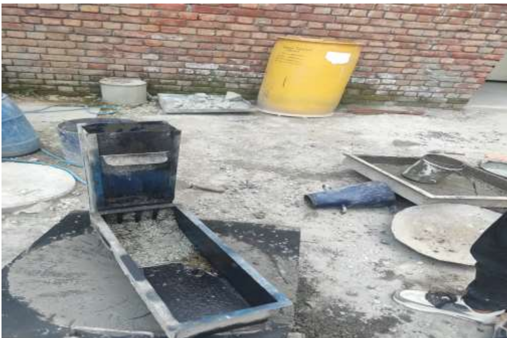
Figure 4.8: L-Box Test Apparatus
