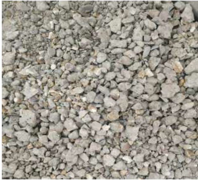
Figure 3.4: Coarse aggregates from demolished concrete for “RCA”
