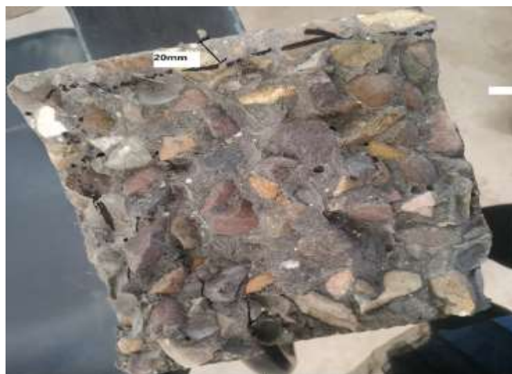
Figure 4.19: Specimen checked for water permeability test
