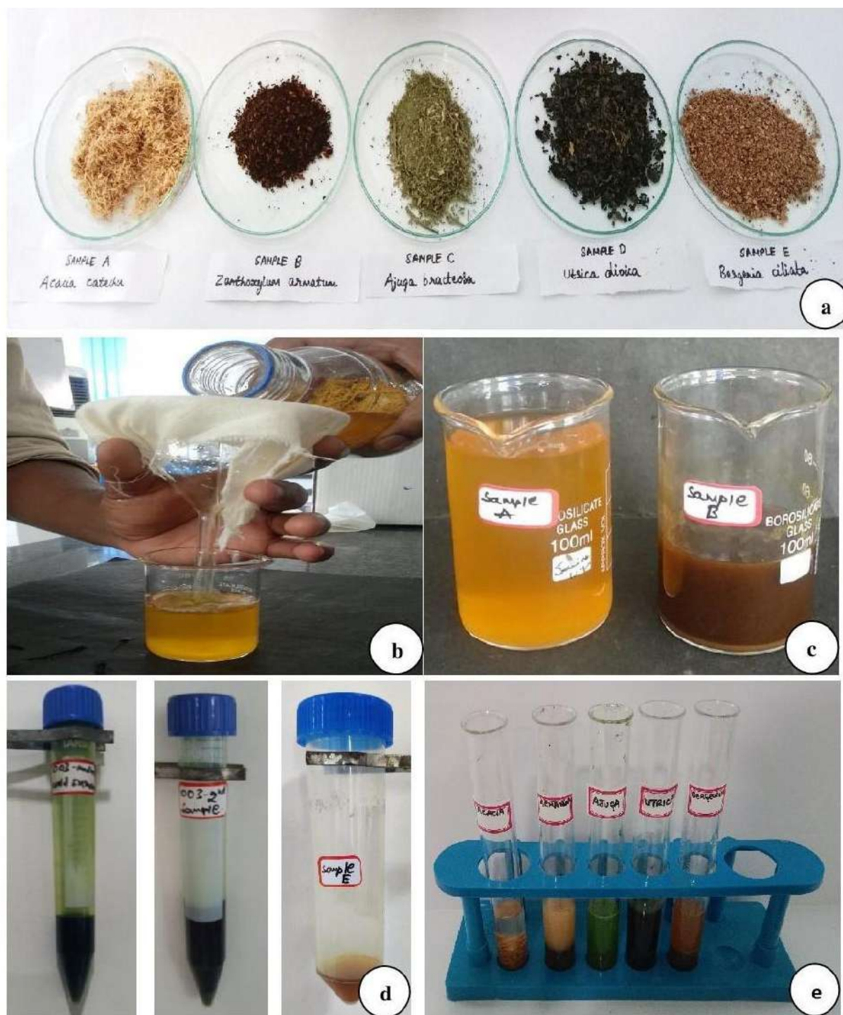
Plate 2(a-e): (a) Shade-dried powdered samples of Acacia catechu heartwood, Ajuga bracteosa leaves, Bergenia ciliata rhizome, Urtica dioica , and Zanthoxylum armatum fruits, (b-e) extraction with different solvents
