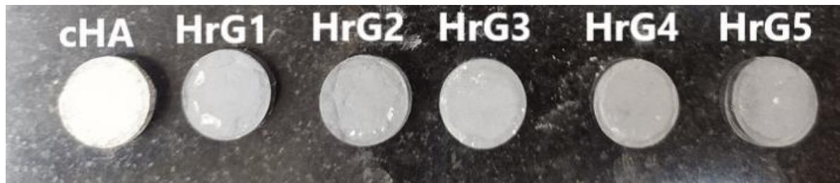
Figure 4.5: Pellets of calcined Hydroxyapatite (cHA) and Reduced graphene oxide (rGO) composites in a different ratio namely HrG1 (90 cHA: 10 rGO), HrG2 (80 cHA: 20 rGO), HrG3 (70 cHA: 30 rGO), HrG4 (60 cHA: 40 rGO) and HrG5 (50 cHA: 50 rGO)
