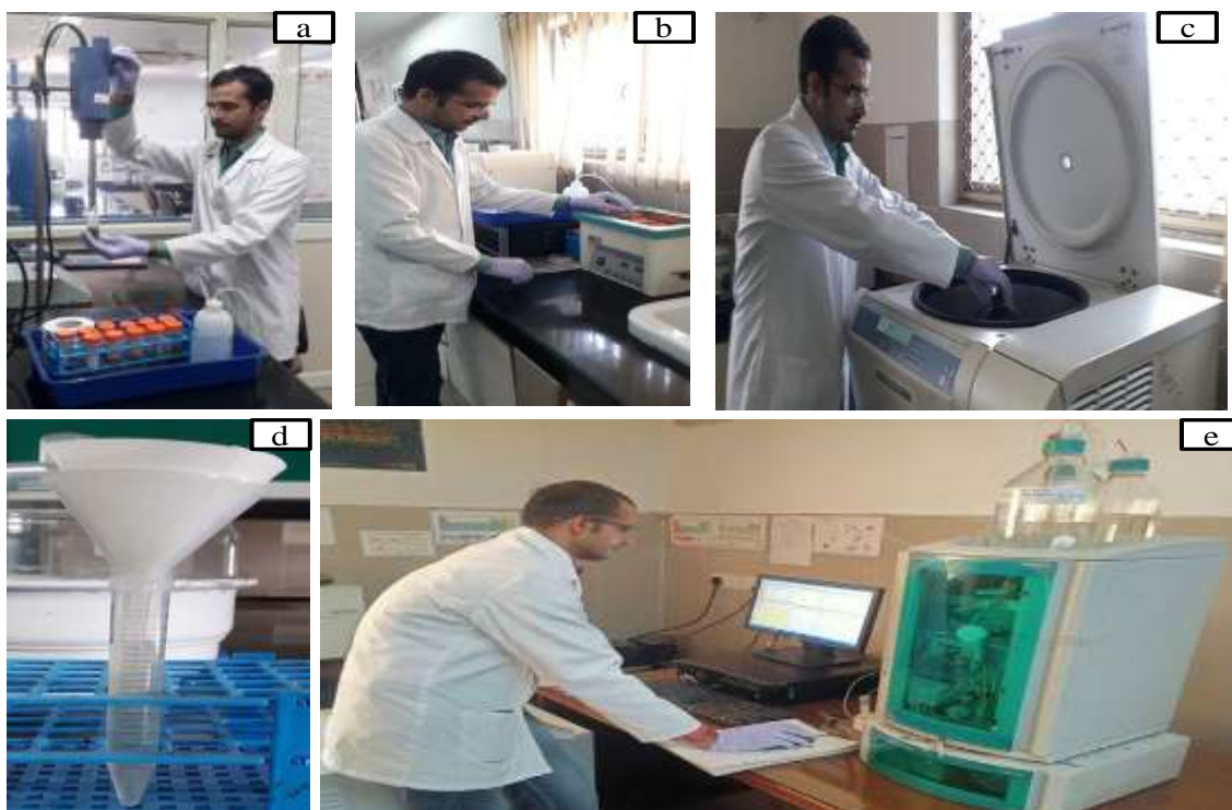
Figure 3.5 (a-e): (a) Homogenization (b) sonication (c) centrifugation (d) filtration (e) ion-chromatography analysis
