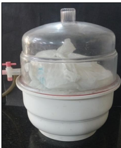
Figure 5.13 Storage of plastic films in the vacuum desiccator. The plastic films were stored in the controlled conditions to avoid any thermal or photo-oxidation
